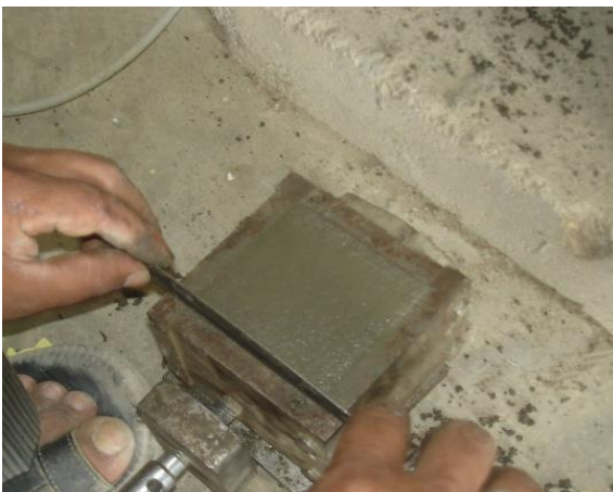
Figure 7: Molding of cement mortar
