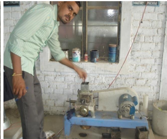
Figure 6: Vibrating the Cement Mortar
