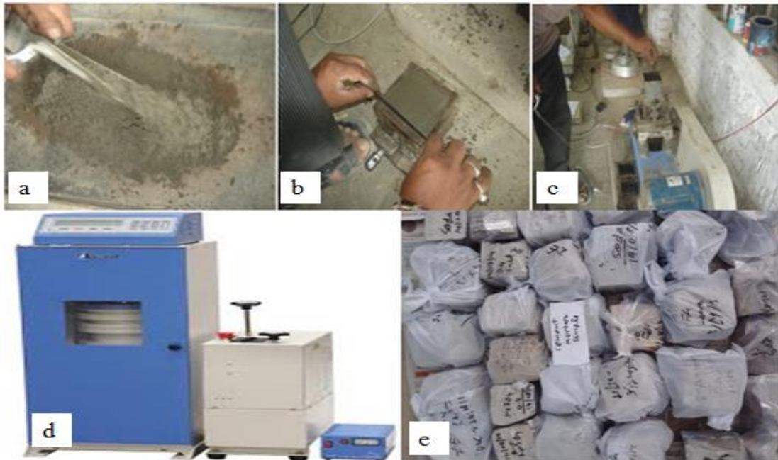
Figure 3.5: About mortar cubes (a) Mixing procedure (b) moulding procedure (c) vibrating machine (d) concrete cubes testing machine (e) tested cubes
