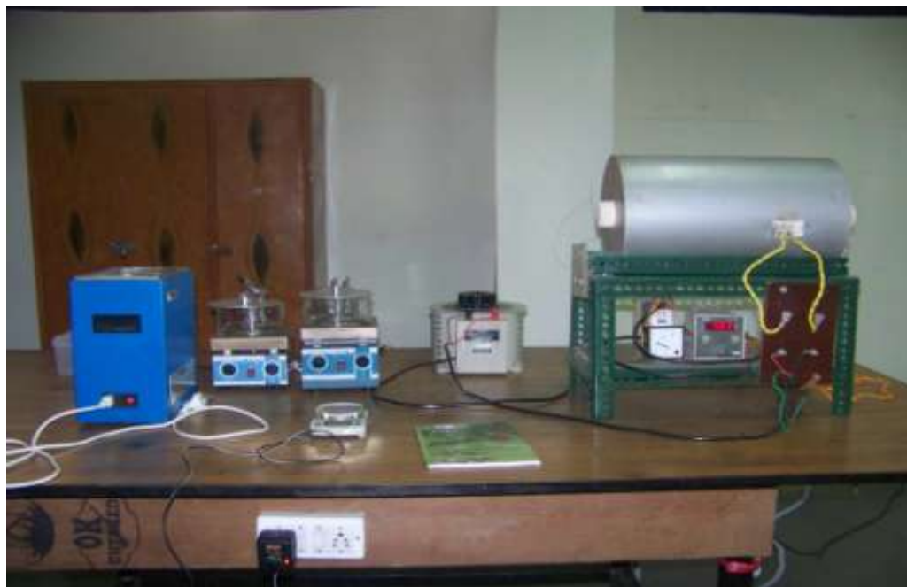
Fig. 3.3: In- house facility for the preparation of sample powders by sol-gel technique and co-precipitation technique setup in the Physics Labs of LPU.
