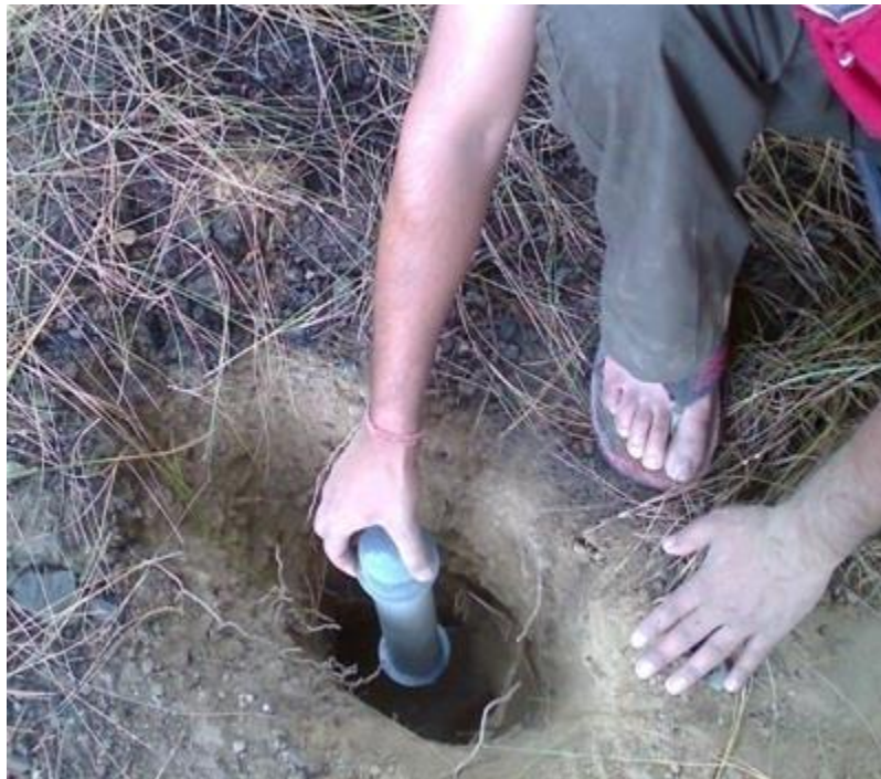
Figure 17: Placement of radon thoron discriminator during soil - gas survey (2)
