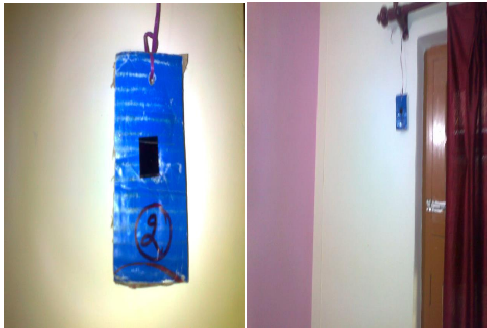
Figure 18: Placement of detector in bare mode for indoor radon survey
