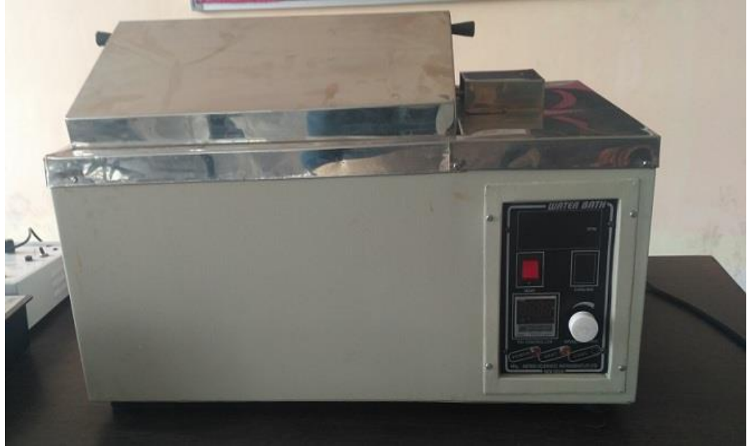
Figure 14: Constant temperature bath and shaker (Etching bath)
