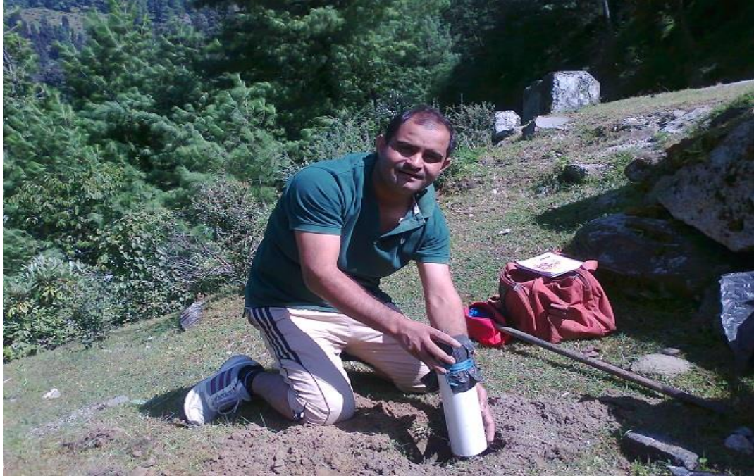
Figure 16: Placement of radon thoron discriminator during soil - gas survey (1)
