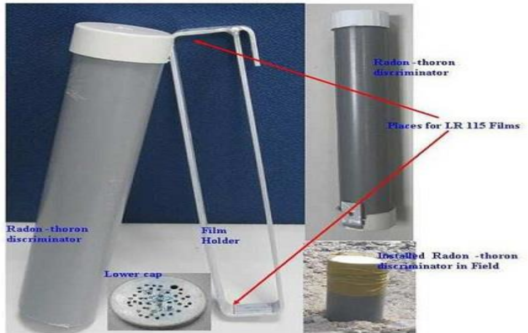
Figure15: Radon-thoron discriminator (Plastic cane with side cap including LR-115 films at the top of the cane and at the bottom of the cane)
