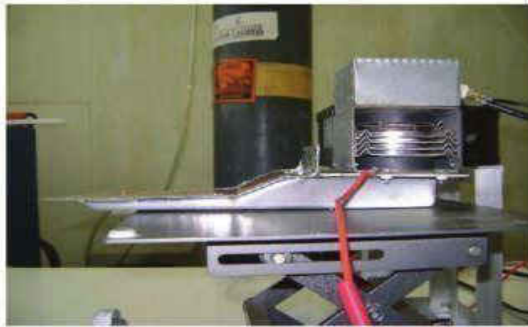
Figure.10 (Magnetron attach with wave guide)
