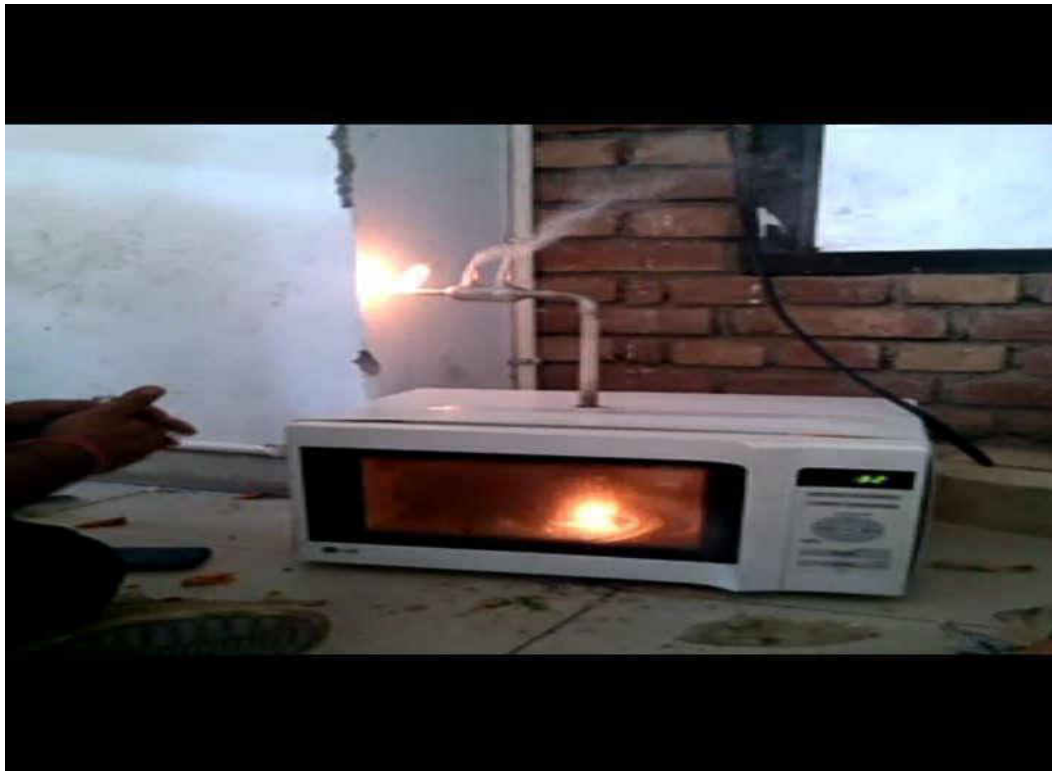
Figure. 6 (Gasification of Domestic waste in cavity of Microwave)
