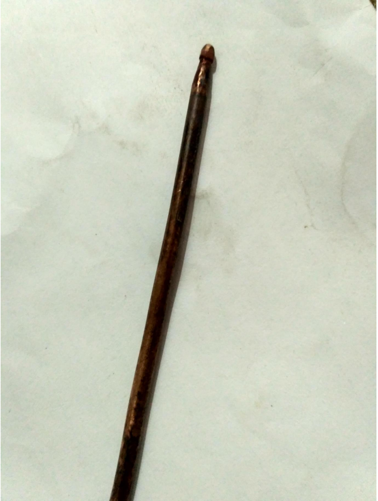
Figure 7 Copper electrodes with spherical shape on its tip
