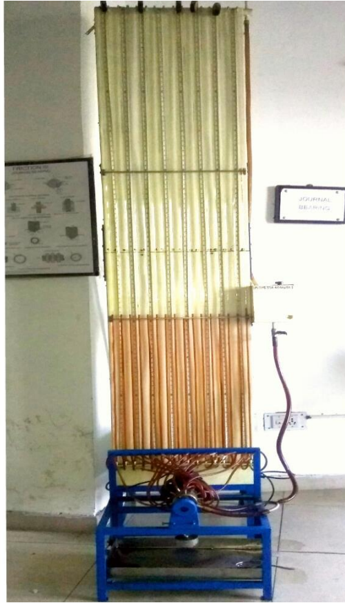
Fig.10 journal bearing setup
