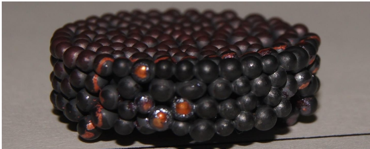
Figure 9 (oxidation layer present in sample 4)
