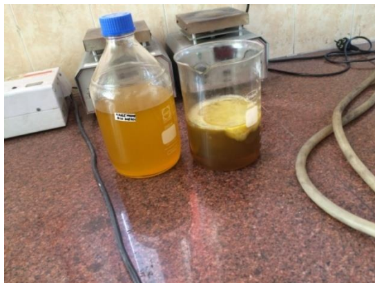
Figure 10 Separation of glycerol after transesterification process
