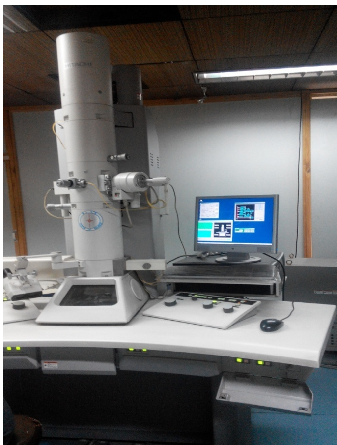
Figure 5.4: Transmission Electron Microscopy (TEM) installed at SAIF LAB Punjab University (Chandigarh) (Model no. Hitachi H-7500)
