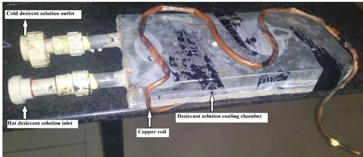
Figure 18: Photograph of desiccant solution cooling chamber
