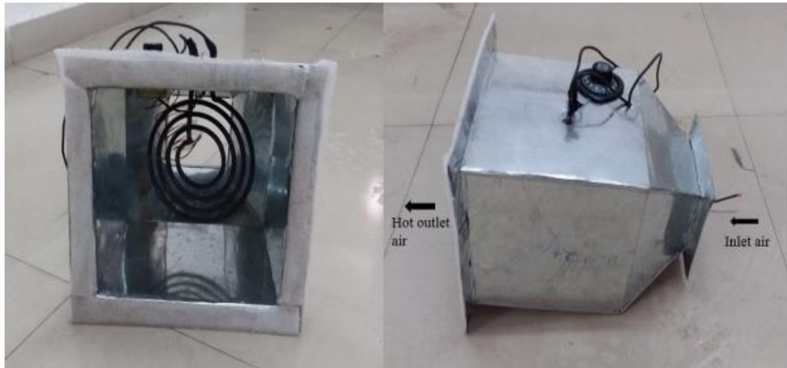
Figure 21: Photograph of air heater
