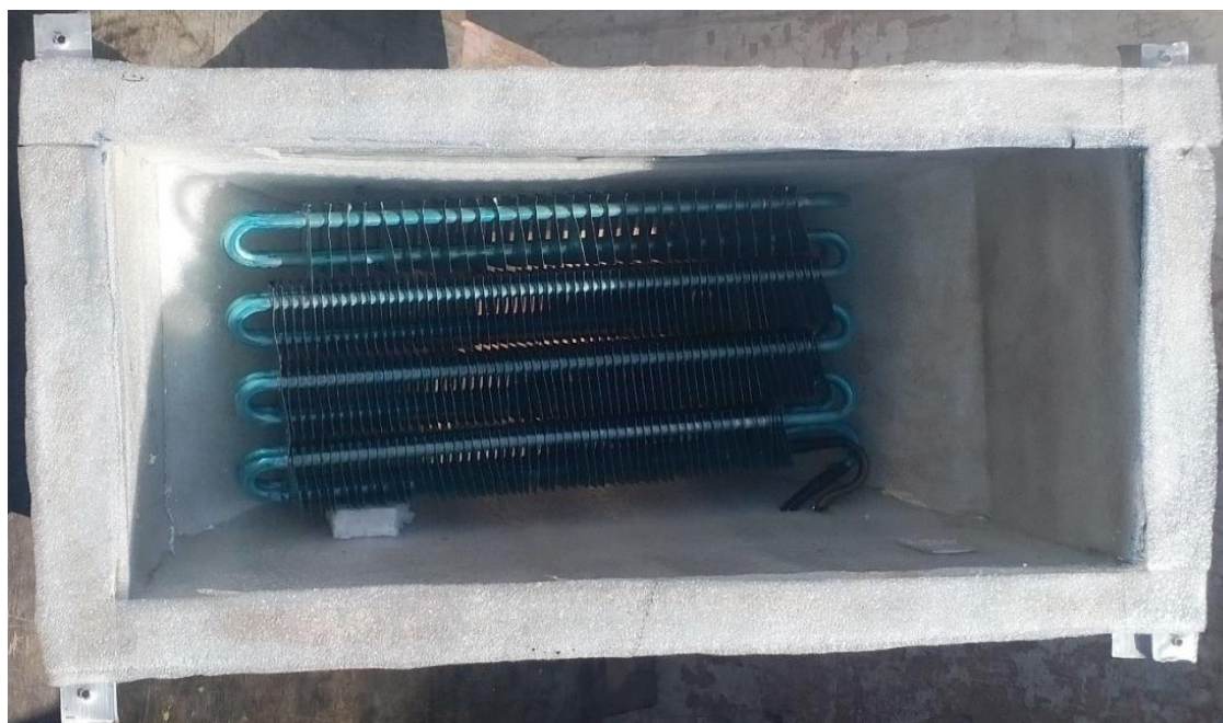
Figure 25: Photograph of arrangement of evaporator coil in the outlet duct of dehumidifier
