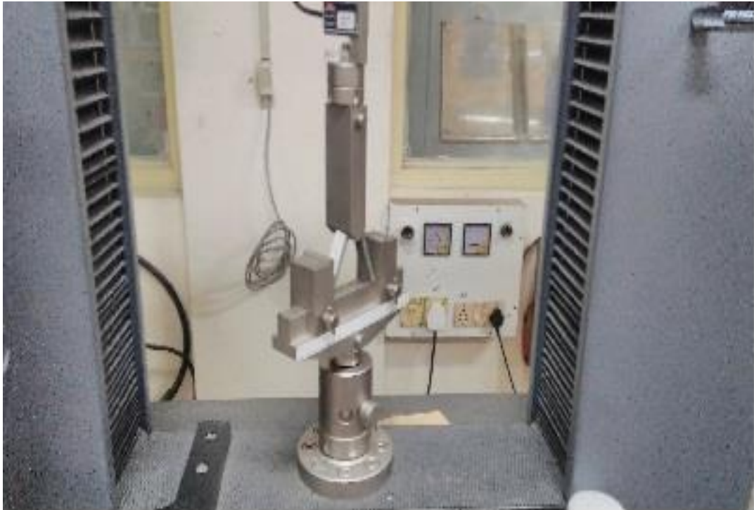
Figure 4.4 Sample break due to applied load in 3 point bending test
