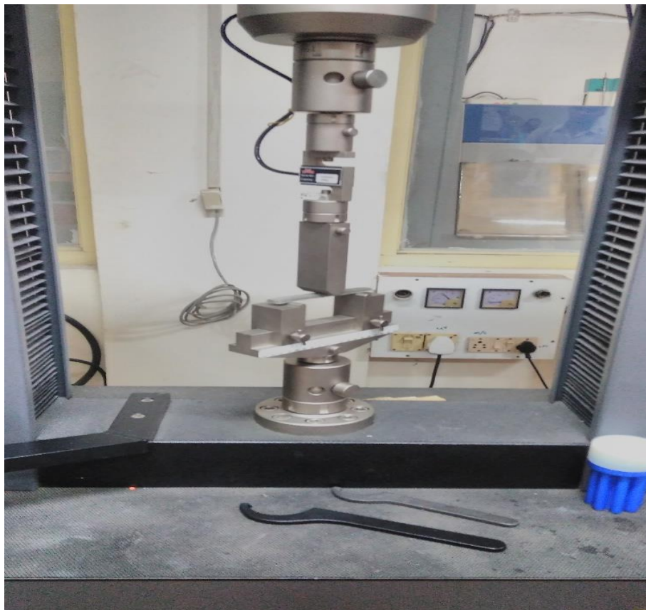
Figure 4.3 Before loading condition in 3 point bending test
