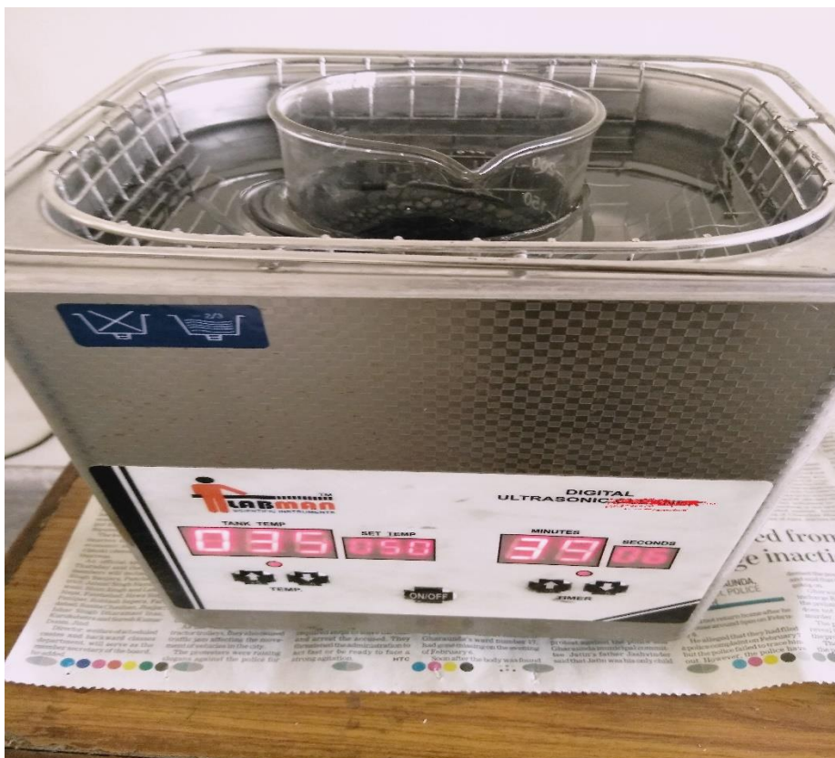
Figure 3.4 Ultrasonic wave mixer from Labman scientific instrument used for MWCNT mixing (courtesy NIT Jalandhar)
