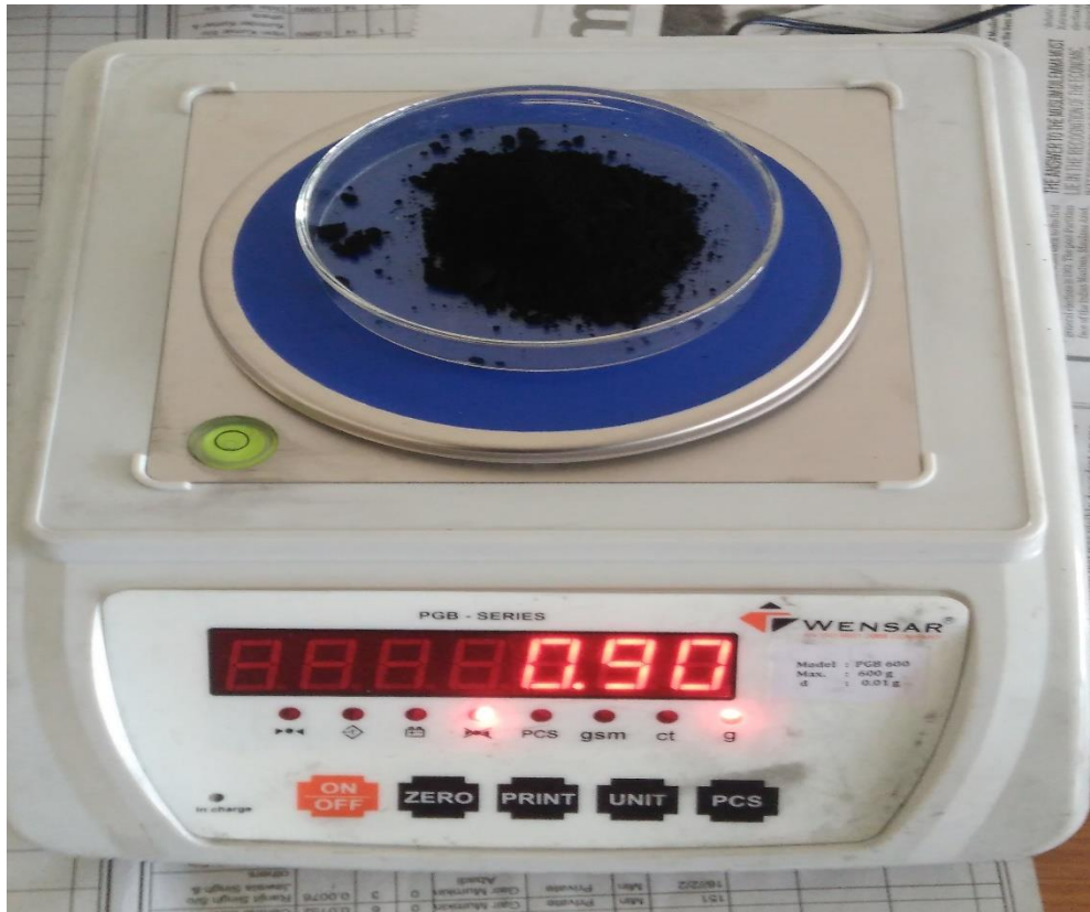
Figure 3.3 Precise scale is used to weigh MWCNTs (courtesy NIT Jalandhar)
