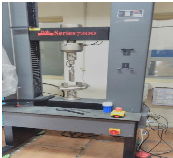
Figure 4.1 Three point bending machine used for testing (courtesy CIPET Amritsar)
