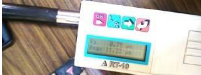
Figure 6 Surface roughness measurement setup
