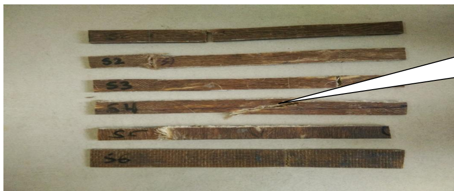
Figure 18: Tensile Test Samples after Testing
