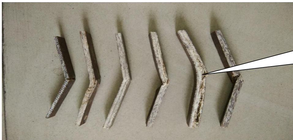
Figure 21: Flexural Test Samples after Testing
