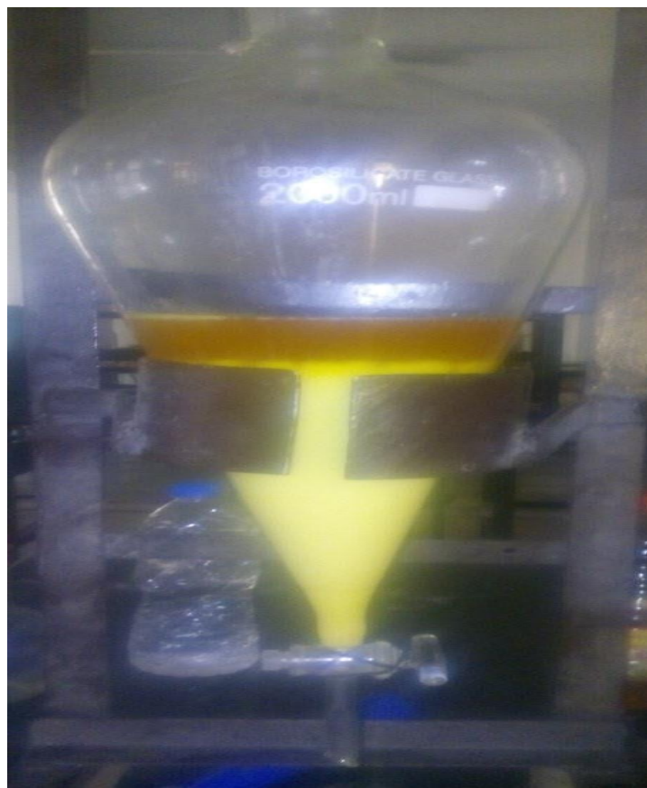
Figure 11: Separation of two layers in separatory Funnel after 1 hour when pouring warm water
