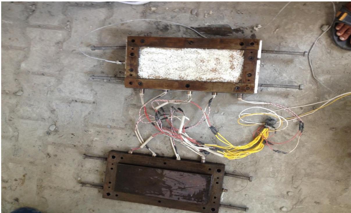
Figure 34 Sprinkling the second layer
