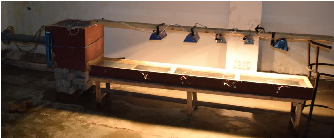
Figure 5.4: Pictorial view of solar air duct
