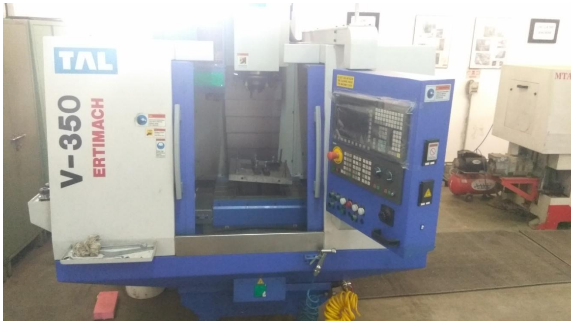
Fig. 5: TAL V-350 CNC Vertical Milling Machine with Fixture
