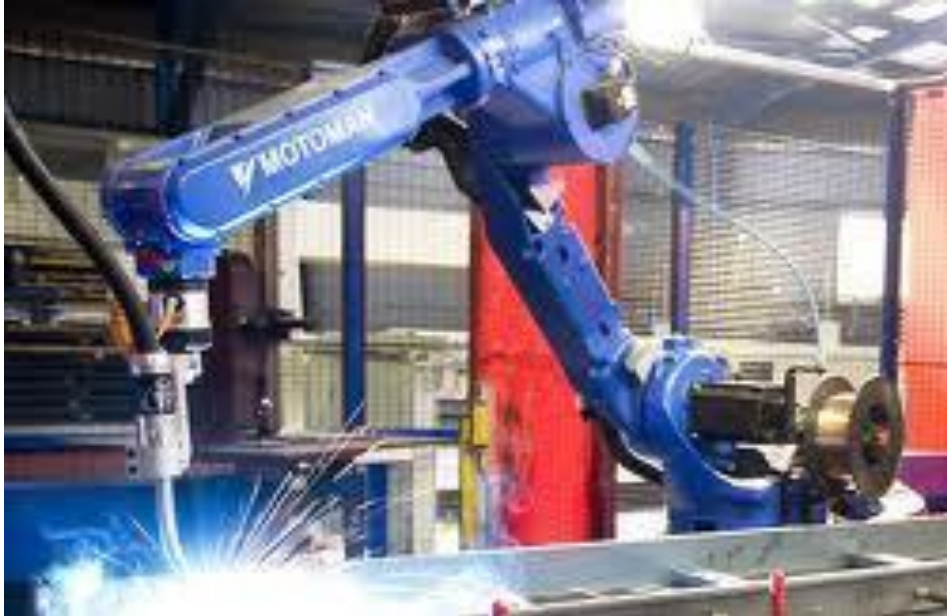
Figure 1.2 Robots used for welding operation
