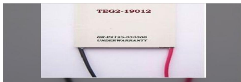
Fig (5) Thermoelectric Generator.
