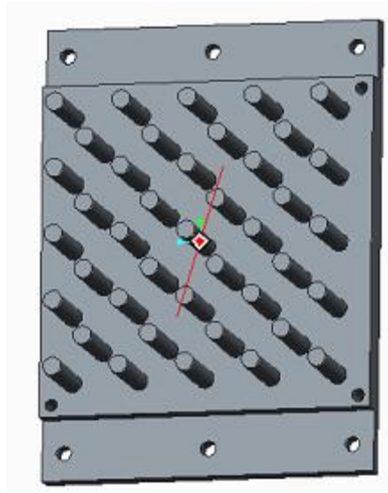
Fig (13) Staggered arrangement of pin-fin absorber
