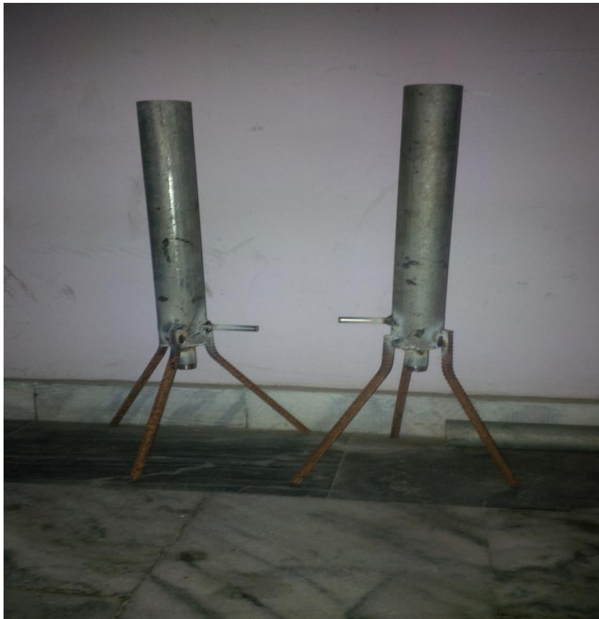
Figure : 1.8 Absorption column and Distillation column(Stripper)
