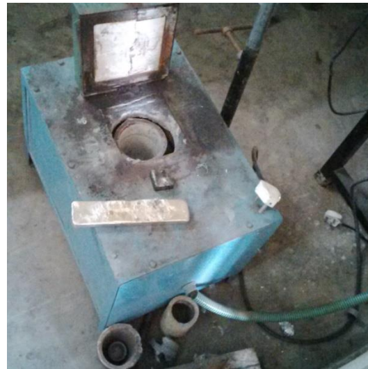
Fig 5: Electrical furnace for melting Aluminum
