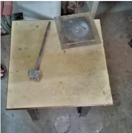
Fig 4: Stirrer used for mixing CNT in Al matrix
