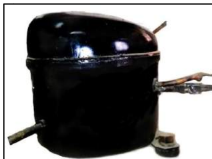
Figure 3. Convection Compressor compatible with R-134a
