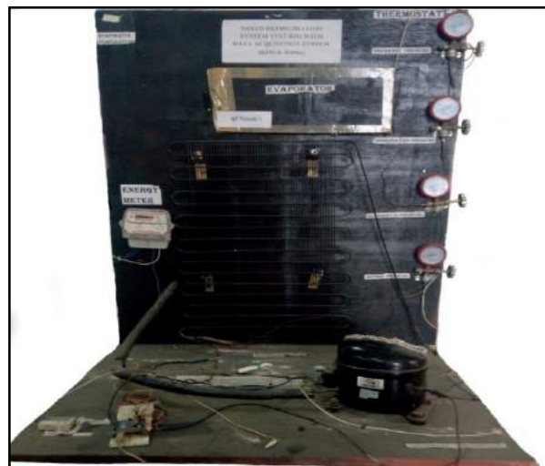
Figure 1. Experimental setup of Vapour Compression Refrigeration System
