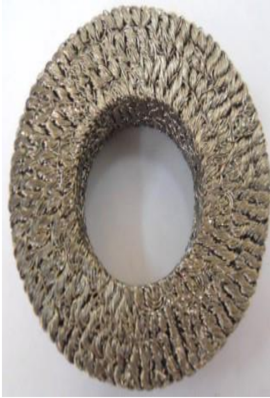
Figure 19: Rubber Isolator, Metal Rubber Isolator
