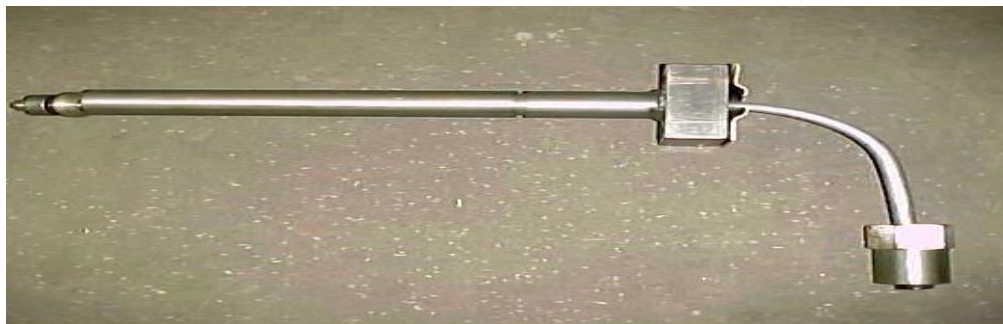
Figure 13H.p tube of FIP pump (rly dsl shed ldh)
