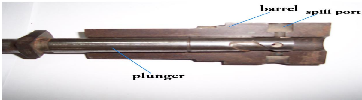
Figure 6. fip pump plunger and barrel
