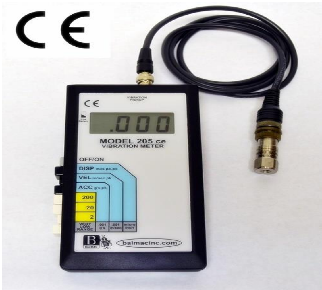
Figure 16 :Vibration Meter (rly dsl shed Idh)
