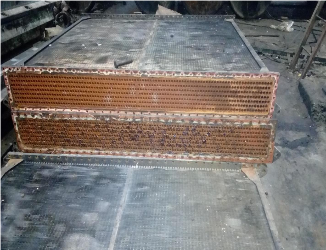
Figure 21: Tube Fin Type Heat Exchanger Courtesy (Indian Railway Diesel Shed Ludhiana)
