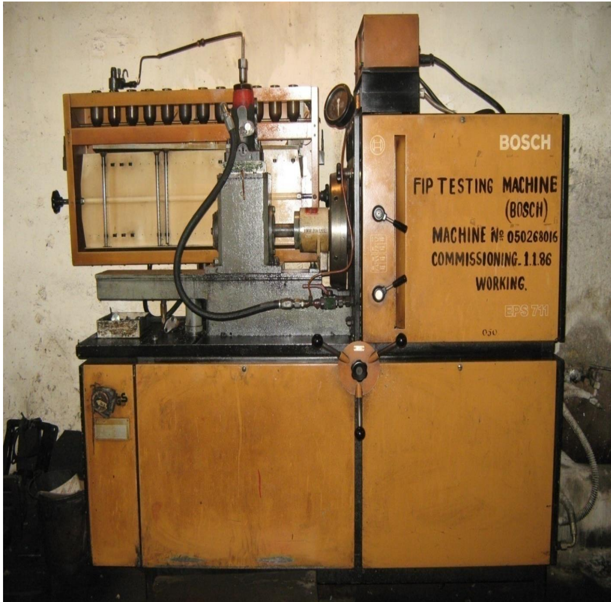
Figure 10 Fip testing machine (rly dsl shed ldh)
