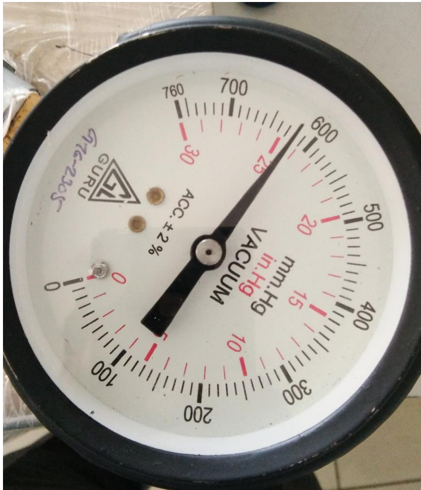
Figure 19 Reading of vacuum pressure after 10 min from start of experiment
