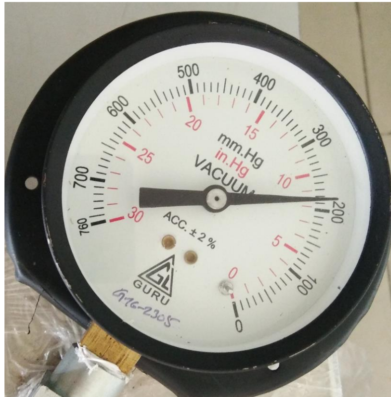
Figure 22 vacuum gauge reading after 40 minutes
