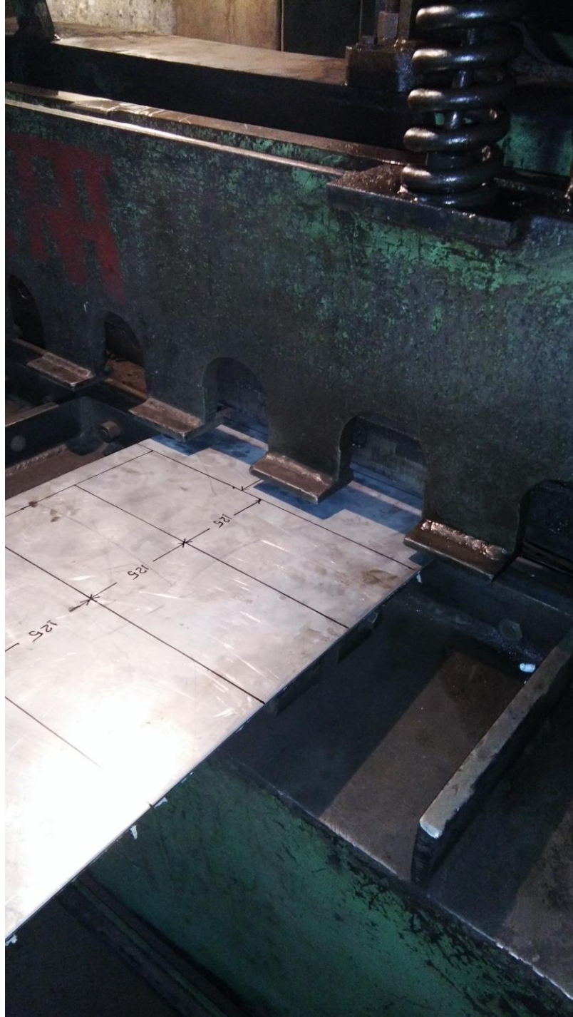
Figure 6 Cutting of SS316 sheet on shearing machine
