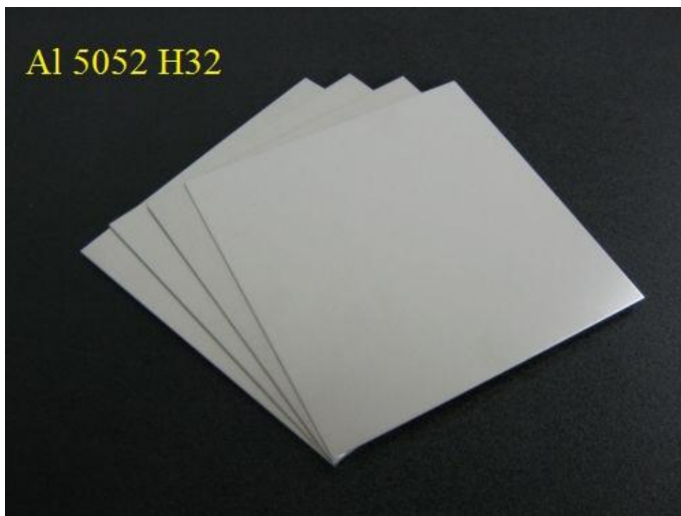
Figure 4 Al5052 - H32 Sheets
