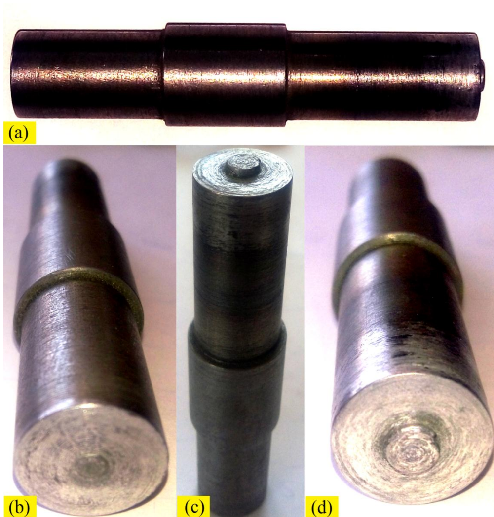
Figure 3 M2 HSS Tool Used For Friction Stir Welding
