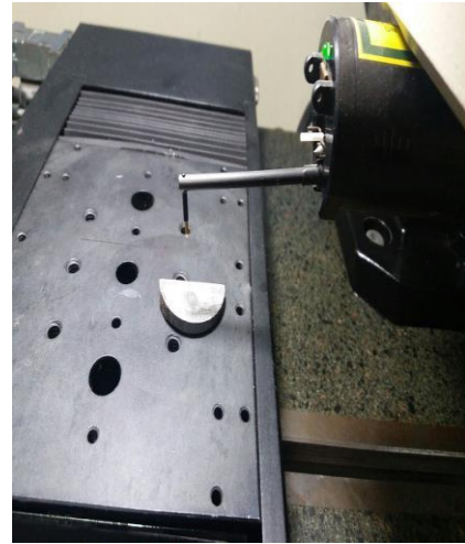
Figure 3.11: Surface roughness of aluminium boron carbide by using Mechanical contact profiler
