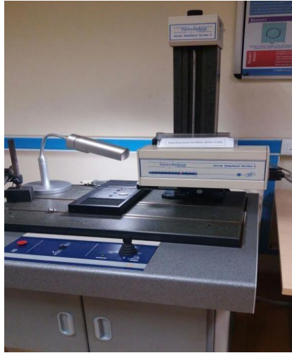
Figure 3.11: Surface roughness of aluminium boron carbide by using Mechanical contact profiler
