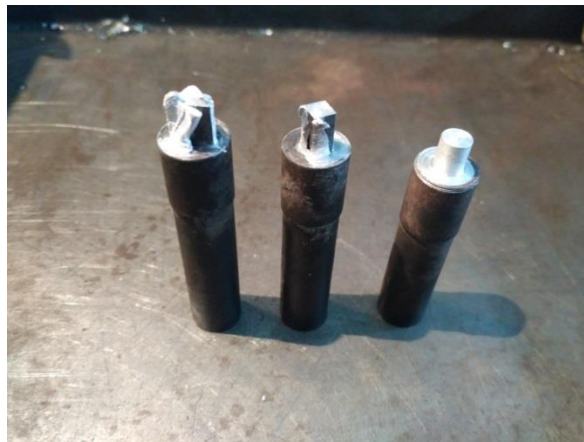
Fig. 6.3: Schematic diagram of tool with square pin of 8 mm diameter and a shoulder diameter of 12 mm
