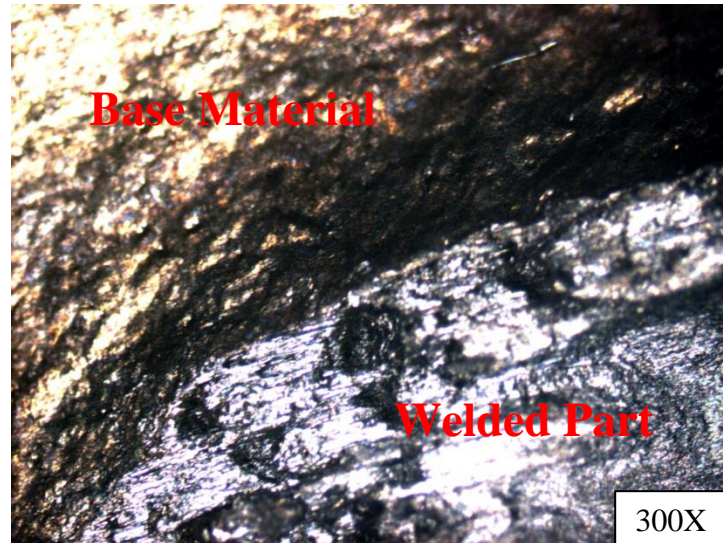
Fig. 9.6 Micro structure of FSSW with square tool at 900 RPM rotational speed and 45 sec dwell time
