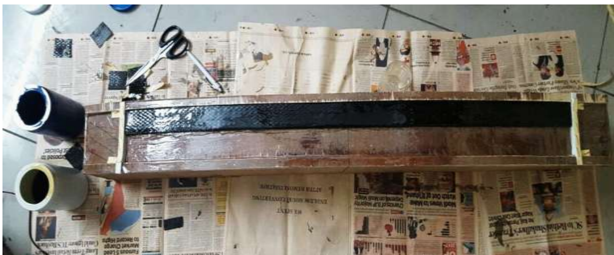
Fig. 6.15. Curing of Composite Mono Leaf Spring
