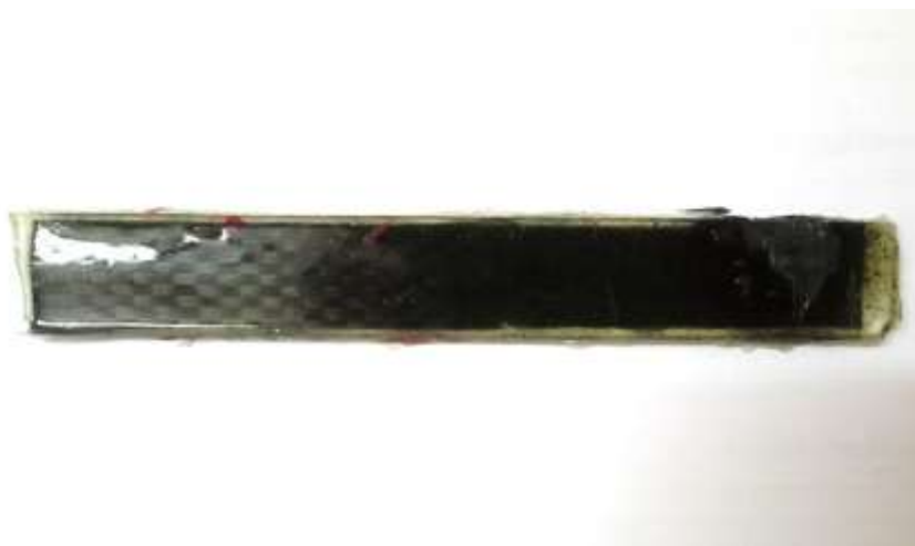
Fig. 6.11. Carbon Fibre Epoxy (Unidirectional) Flexural Test Specimen ASTM D-7264
