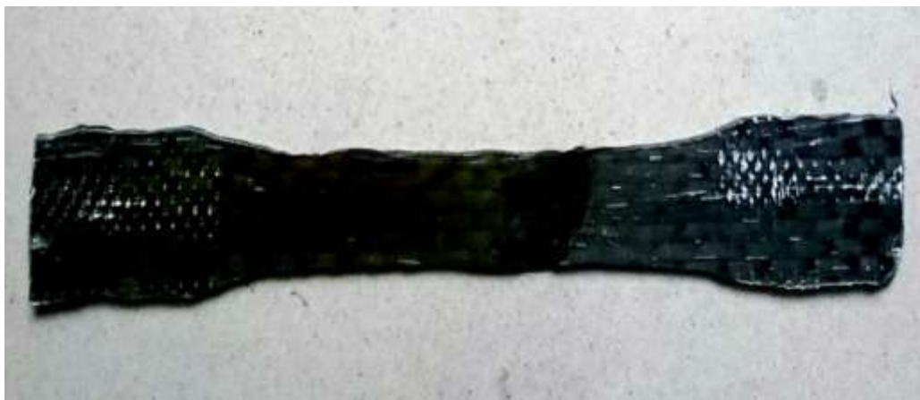
Fig. 6.7 Unidirectional carbon-glass fibre epoxy specimen (ASTM D638 TYPE-I Tensile Bar)
