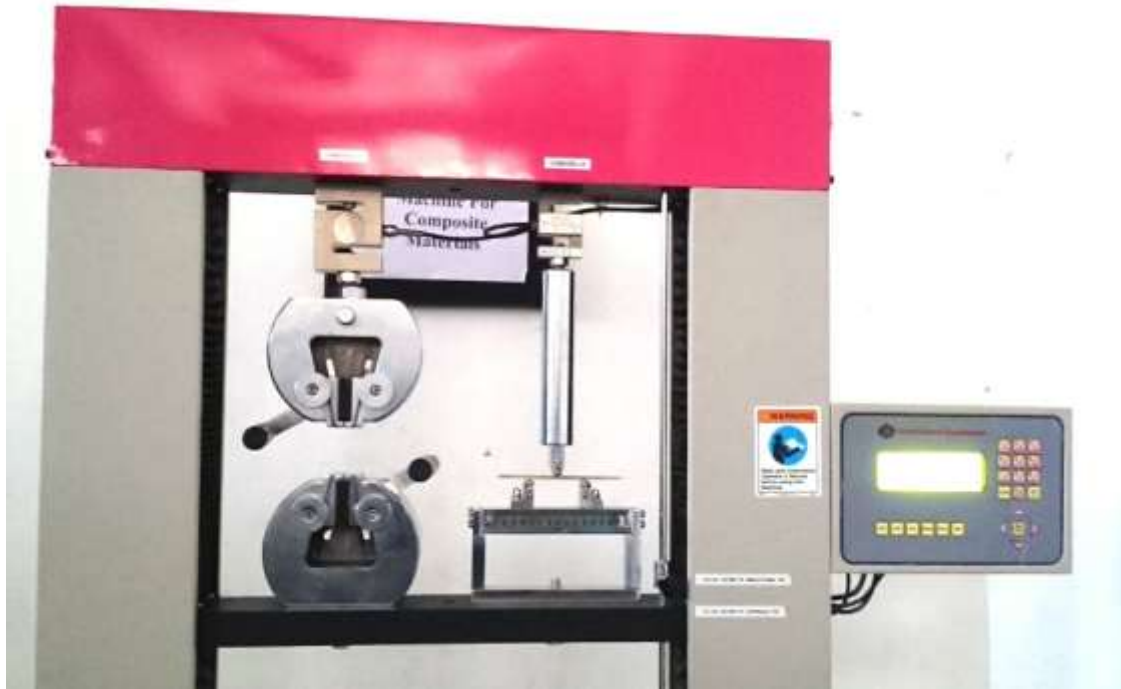
Fig. 8.7. Flexural Testing for composite materials.
