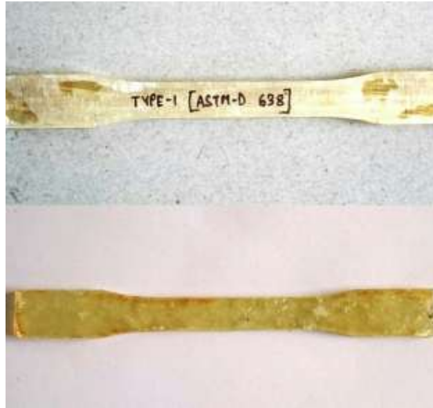
Fig. 8.2 ASTM D 638 type I Tensile Bar Specimen for Fibre Glass
