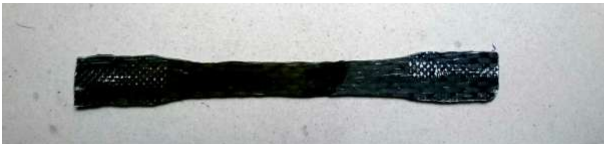
Fig. 8.4 ASTM D 638 type I Tensile Bar Specimen for carbon-glass fibre epoxy
