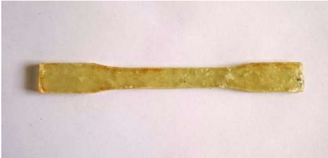
Fig. 6.8. (RANDOM) Fibre glass epoxy specimen (ASTM D638 TYPE-I Tensile Bar)
