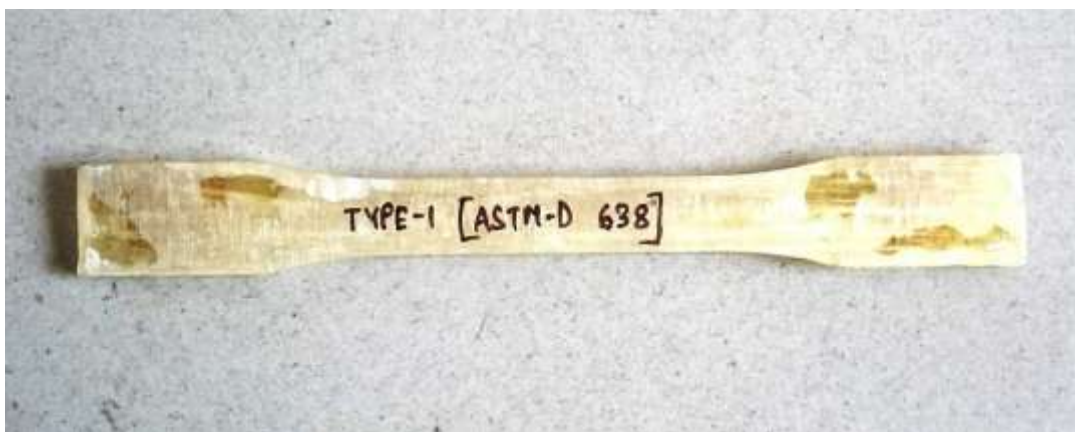
Fig. 6.5. (Unidirectional) Fibre Glass Epoxy Specimen (ASTM D638 TYPE-I Tensile Bar)
