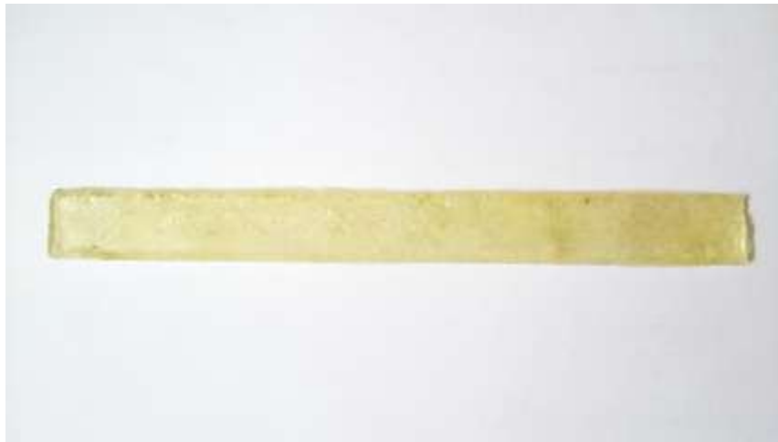
Fig. 6.10. Fibre Glass Epoxy (Unidirectional) Flexural Test Specimen ASTM D-7264
