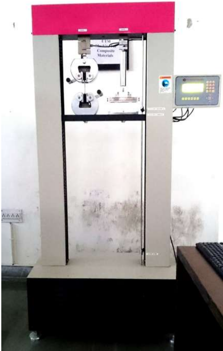
Fig. 5.1. Universal Testing Machine for composite
