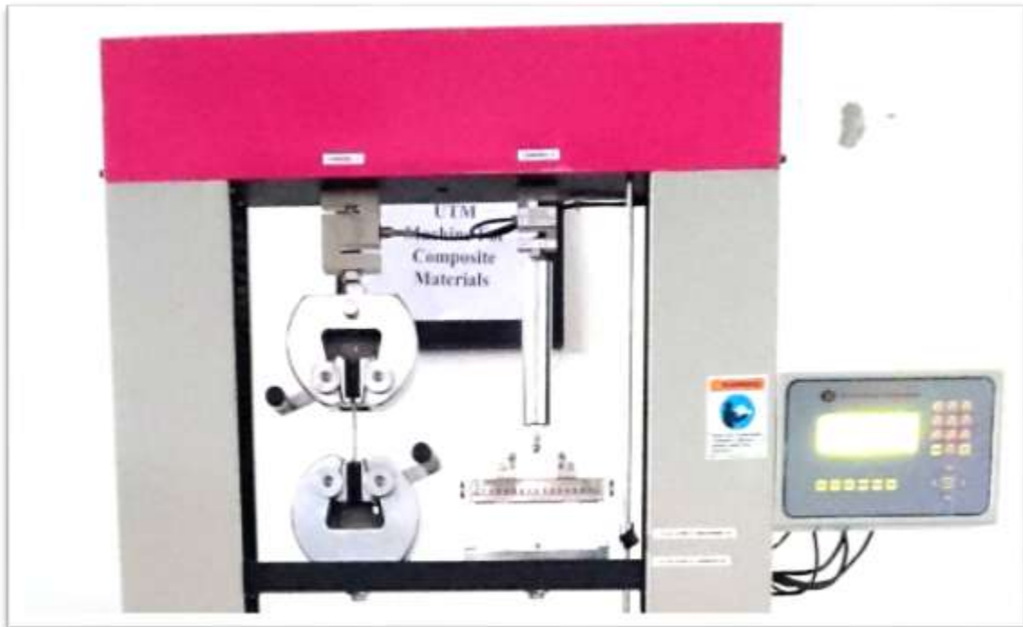
Fig. 8.6. Tensile Testing for composite materials.
