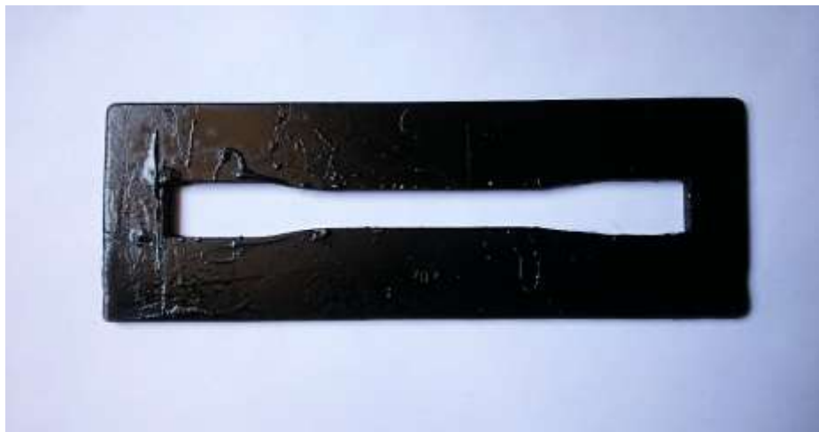
Fig. 6.3. Mild steel die for specimen preparation
