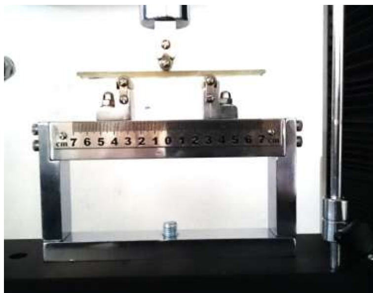
Fig. 6.13. 3-Point flexural test support span
