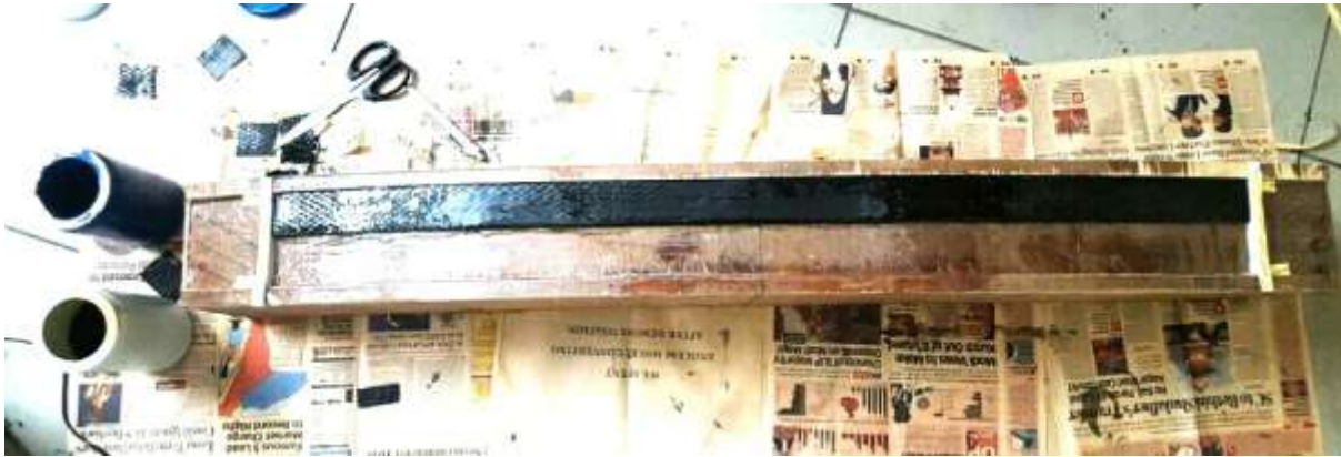
Fig. 8.11. Hand Lay-up Method (composite leaf spring)
