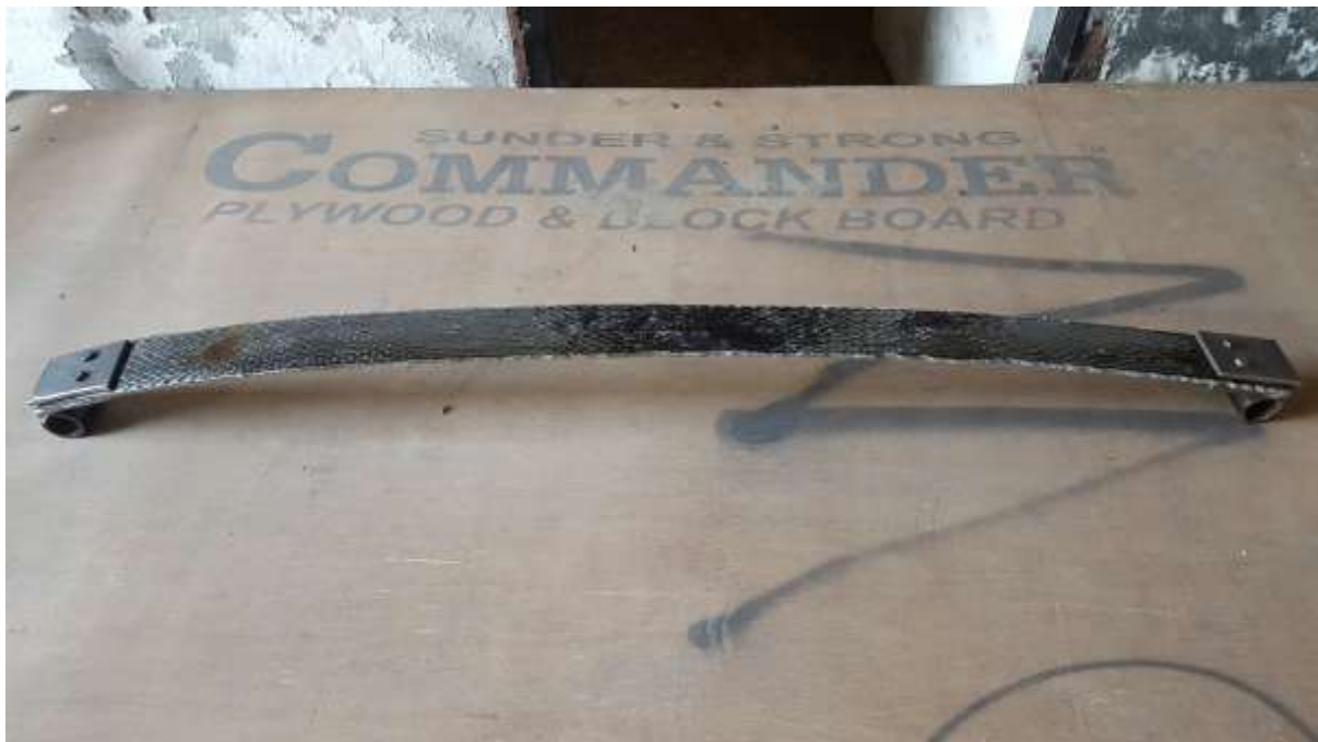
Fig. 8.13. Carbon fibre Epoxy Leaf Spring
