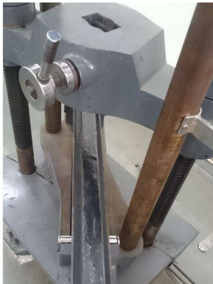
Fig. 6.19 Carbon Fibre Epoxy Mono leaf spring under UTM for testing
