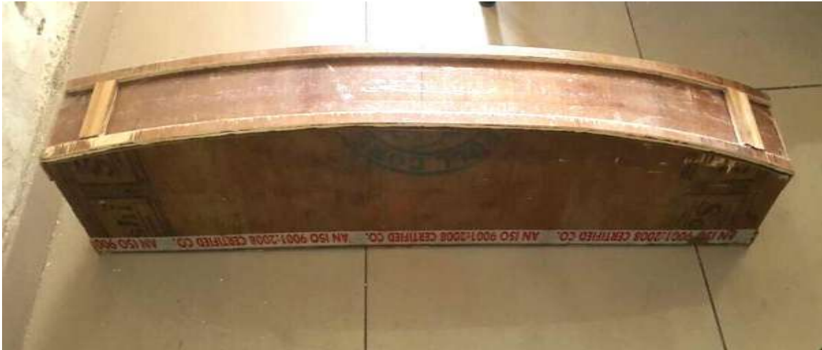
Fig. 6.14. Prepared mould for composite leaf spring.
