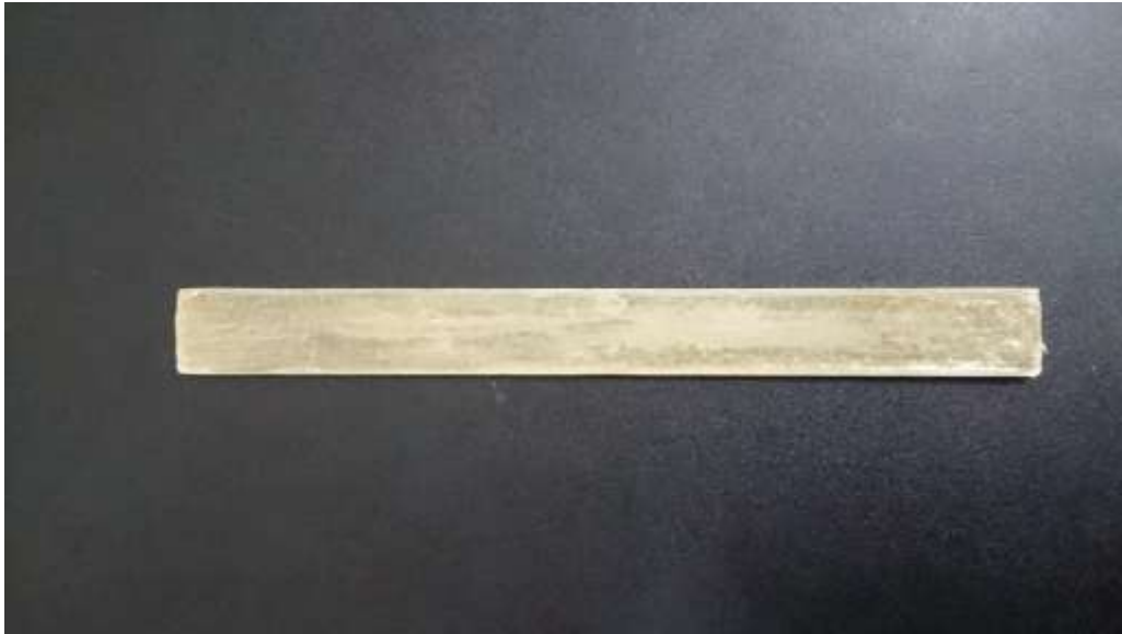
Fig. 8.5. Flexural Test Specimen
