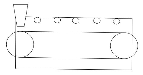
Diameter of one mould is 9cm Space between two moulds is 4cm Length of the conveyor is 500cm Breadth of the conveyor is 100cm With the diameter of mould 9cm and blank space between two moulds 4cm, one mould acquire 13cm area.
