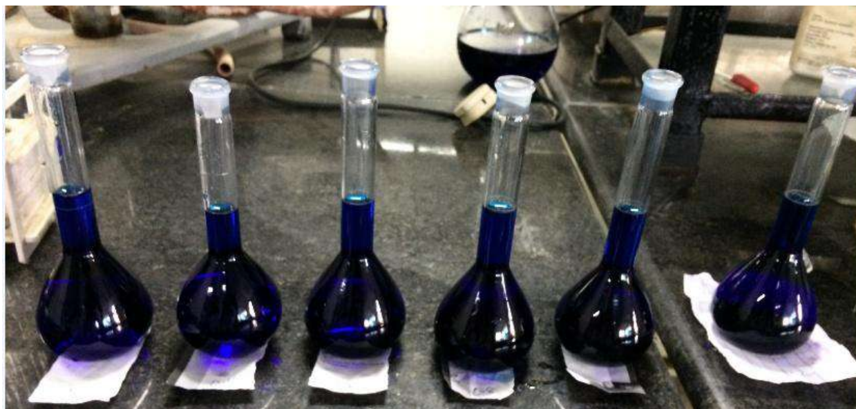
Figure 2: Preparation of solution of Methylene blue with activated carbon
