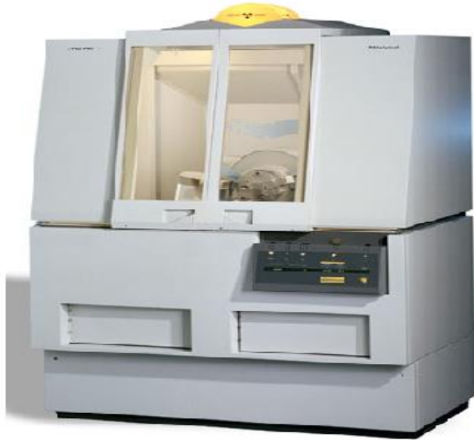
Fig 3.3 The above diagram shows the X' Pert PRO, PANalytical apparatus for obtaining XRD patterns [29]
