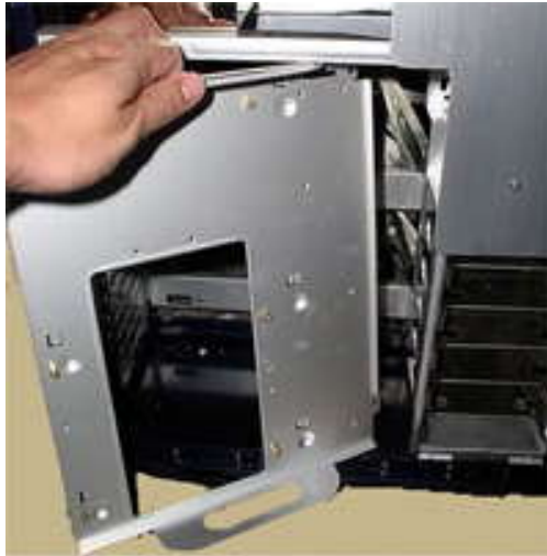
Figure 3.7: Removing Motherboard Tray
