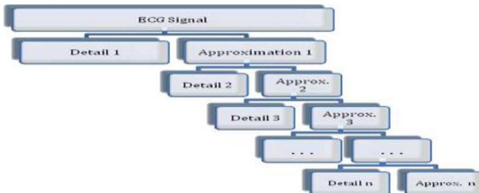
Figure 6.9 Decomposition flow with LPF (Approximation Coefficients) & HPF (Detail Coefficients).
