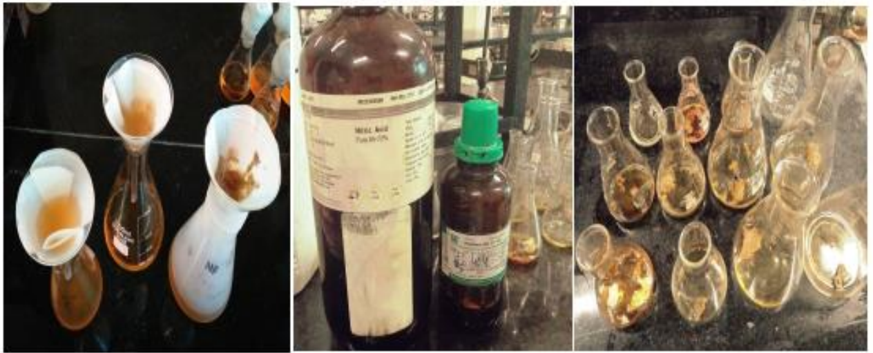
Figure 4.12: Filtration of biomass of Aspergillus flavus and digestion of dried biomass with nitric acid and perchloric acid (3:1)
