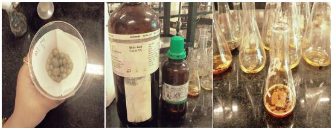
Figure 4.15: Filtration of biomass of Penicillium citrinum and digestion of dried biomass with nitric acid and perchloric acid (3:1)
