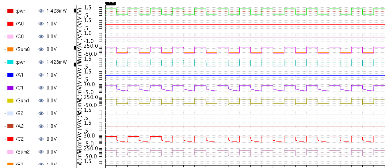
Figure.4.10 Transient Analysis of 8 Bit Full Adder Cell on the combination of GDI and Adiabatic Logic of ECRL
