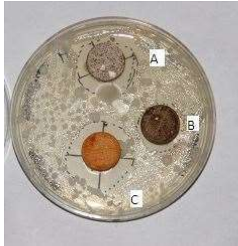
Figure 11. Nutrient Agar Petri Plates with growth of S.aureus having punched out wells carrying wells containing 50% HAP and 50% Amla or Clove or Tumeric ; showing Zones of Inhibition
