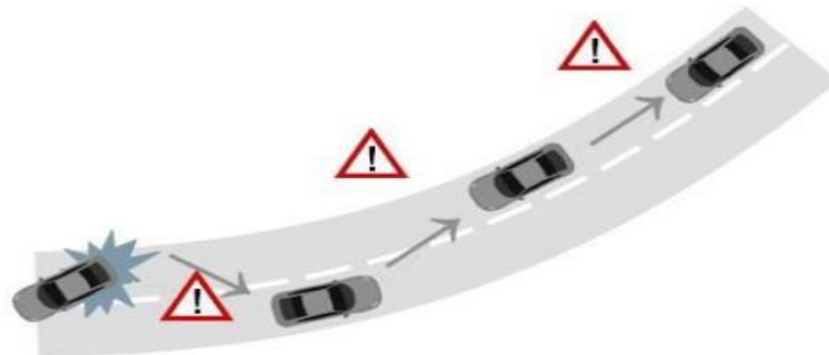
Fig. 1.3 Inter vehicles communications
