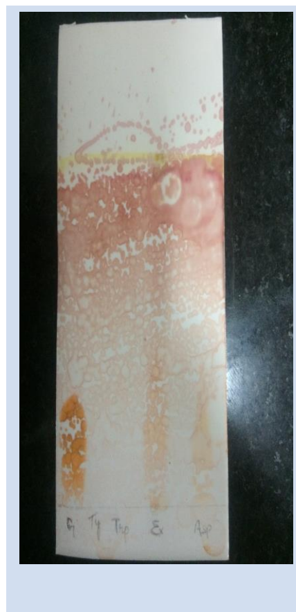
Fig 19: TLC of amino acids on commercial silica plate
