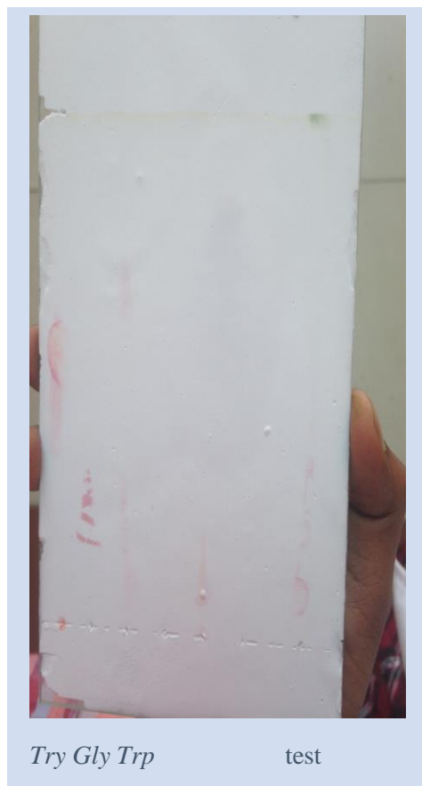
Fig 18: TLC of amino acids on prepared silica plate
