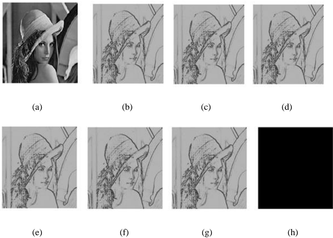
Fig.5.18 (a) original image with edges for thresholds (b) 0.00 (c) 0.01 (d) 0.02 (e) T=0.09 (f) 0.10 (g) 0.20 (h) 0.50
