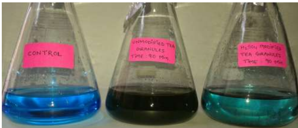
4(c) Dye decolourization by H_2SO_4 modified and unmodified TG and TL after 90 minutes.
