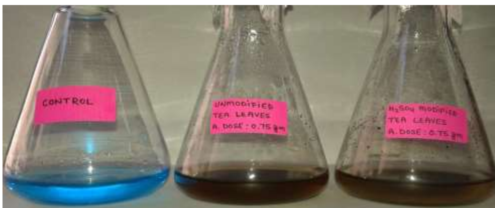
5(c) Dye decolourization by \text{H}_2\text{SO}_4 modified and unmodified TG and TL with adsorbent dose of 0.75 gm.
