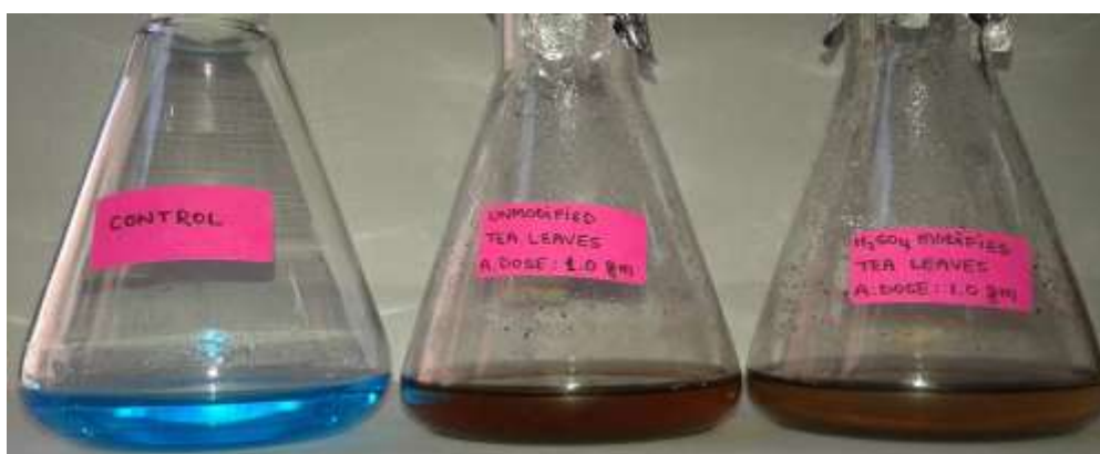
5(d) Dye decolourization by \text{H}_2\text{SO}_4 modified and unmodified TG and TL with adsorbent dose of 1.0 gm.
