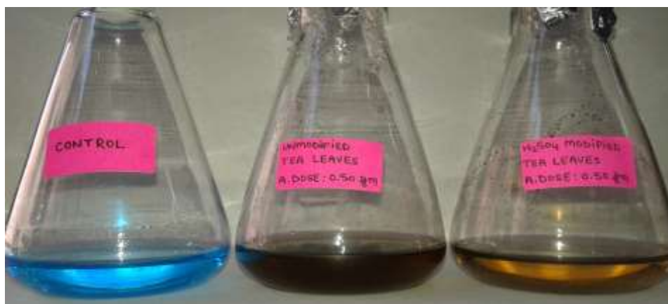
5(b) Dye decolorization by H_2SO_4 modified and unmodified TG and TL with adsorbent dose of 0.50 gm.
