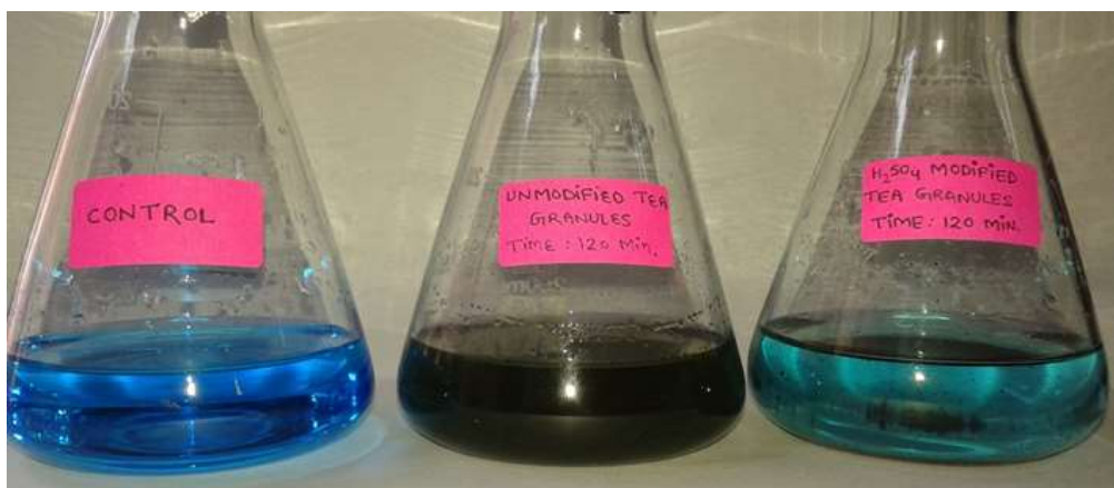
4(d) Dye decolourization by H_2SO_4 modified and unmodified TG and TL after 90 minutes.
