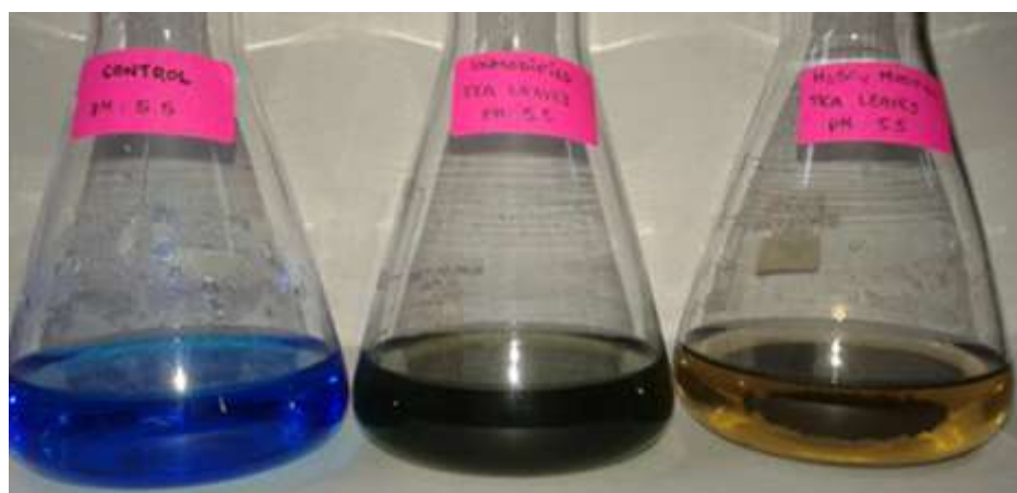
3 (a) Dye decolourization by H 2 SO 4 modified and unmodified TG and TL at pH: 5.5
