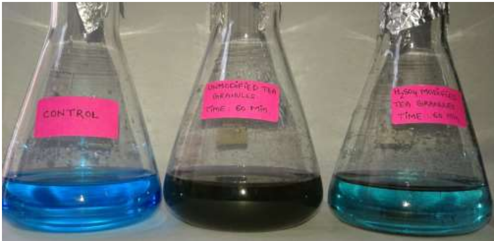
4(b) Dye decolourization by H_2SO_4 modified and unmodified TG and TL after 60 Minutes.
