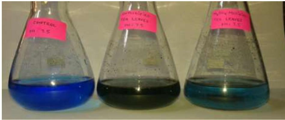
3(c) Dye decolourization by \text{H}_2\text{SO}_4 modified and unmodified TG and TL at pH: 7.5
