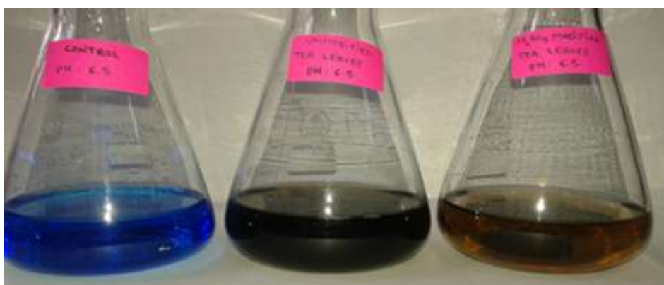
3(b) Dye decolourization by H 2 SO 4 modified and unmodified TG and TL at pH: 6.5
