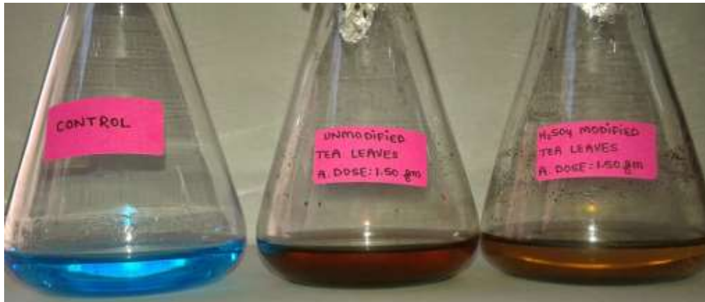
5(f) Dye decolourization by H 2 SO 4 modified and unmodified TG and TL with adsorbent dose of 1.50 gm.
