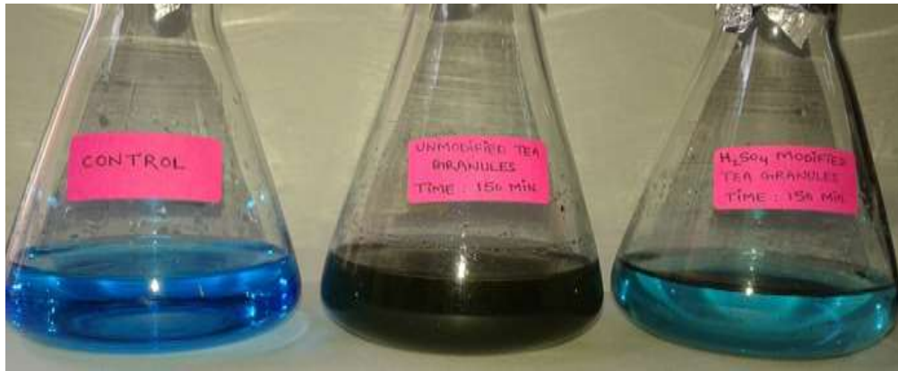
4(e) Dye decolorization by H_2SO_4 modified and unmodified TG and TL after 150 minutes.
