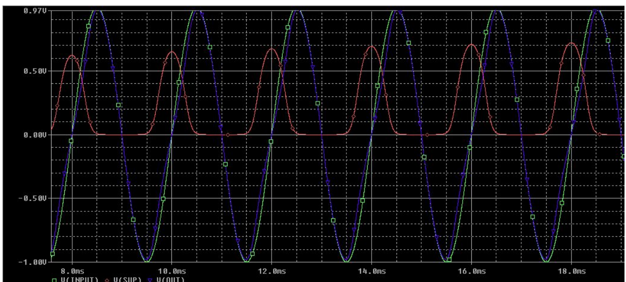
Figure 5.6 : memristor in/out voltage output.
