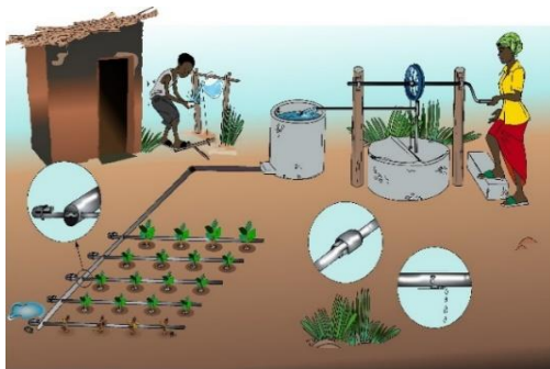
Figure 9: Drip irrigation layout
