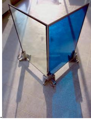
Fig 10 show two glass panels of electrochromic materials (Reece, 2006)
