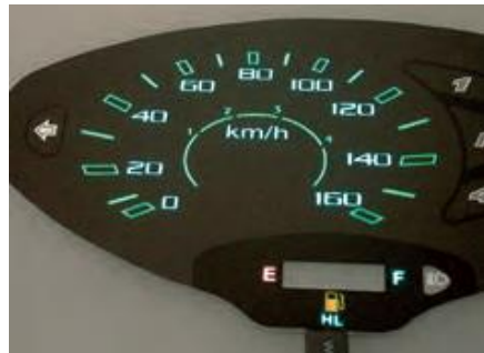
Fig 23 show EL ink on speedometer
