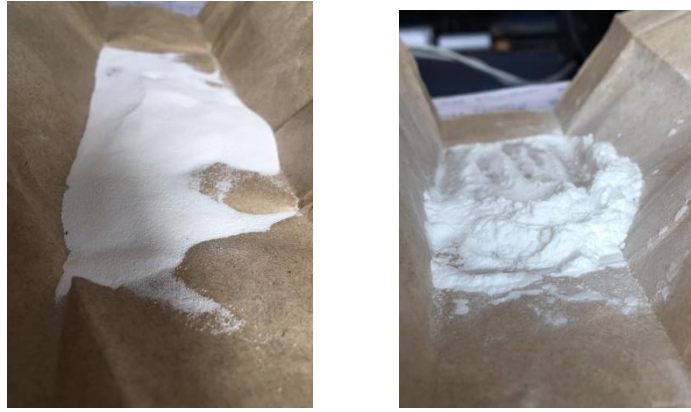
Fig 49 show the chemical compound of a) activated alumina and b) silica gels (Source: author)
