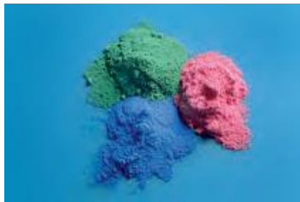
Fig 9 show powdered microencapsulated TCs (Reece, 2006)
