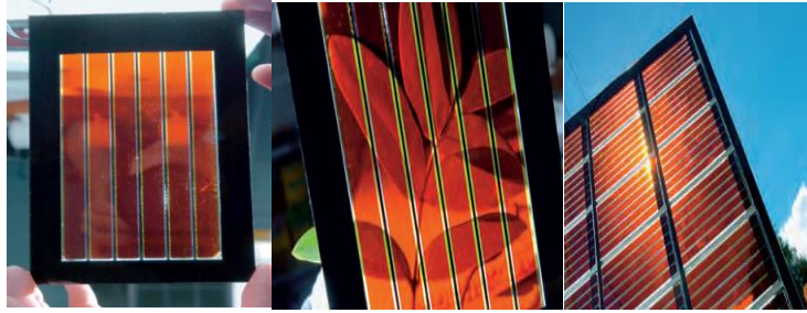
Fig 27 shows six DSC modules and Transparent effect of the dye used (Reece, 2006)
