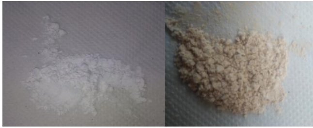
Fig 43 show the real experiment of silver bromide when react with light and heat (Source: author)
