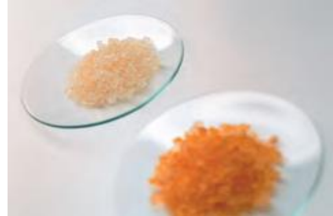
Fig 36 show silica gel granule methyl orange as indicator in active or inactive
