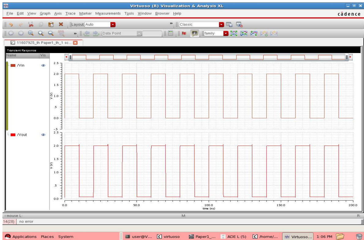
Figure 19: Transient Response for Body biasing based Schmitt trigger Design at V_n=1.2v and V_p=0.5v . It can be analyzed from figure-19 that the body biasing based Schmitt trigger design acts as a buffer. It is also clear that input-output voltage range is also same for the buffer i.e. input is 2V and output is also of same level.
