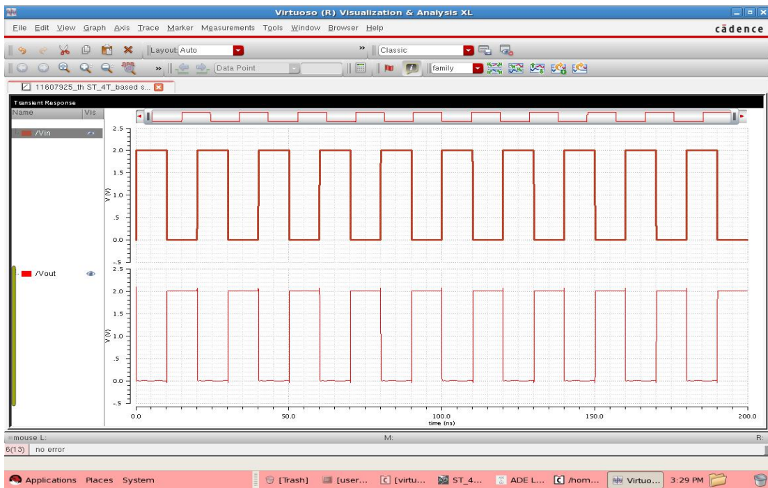
Figure 17: Transient Response for 4T based Schmitt trigger Design using pulse wave as Input
