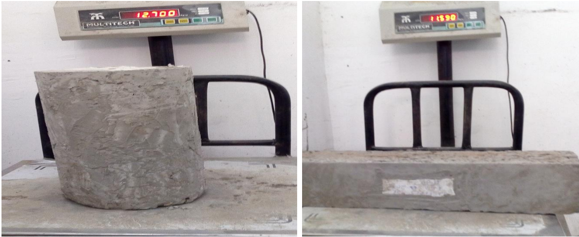
Figure 13: Self-Weight of Normal Concrete (Cylinder & Beam)
