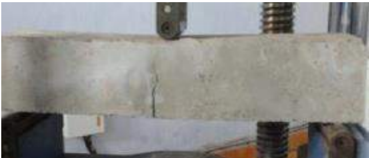
Fig23: Failure of concrete beam (Source: www.ijera.com )
