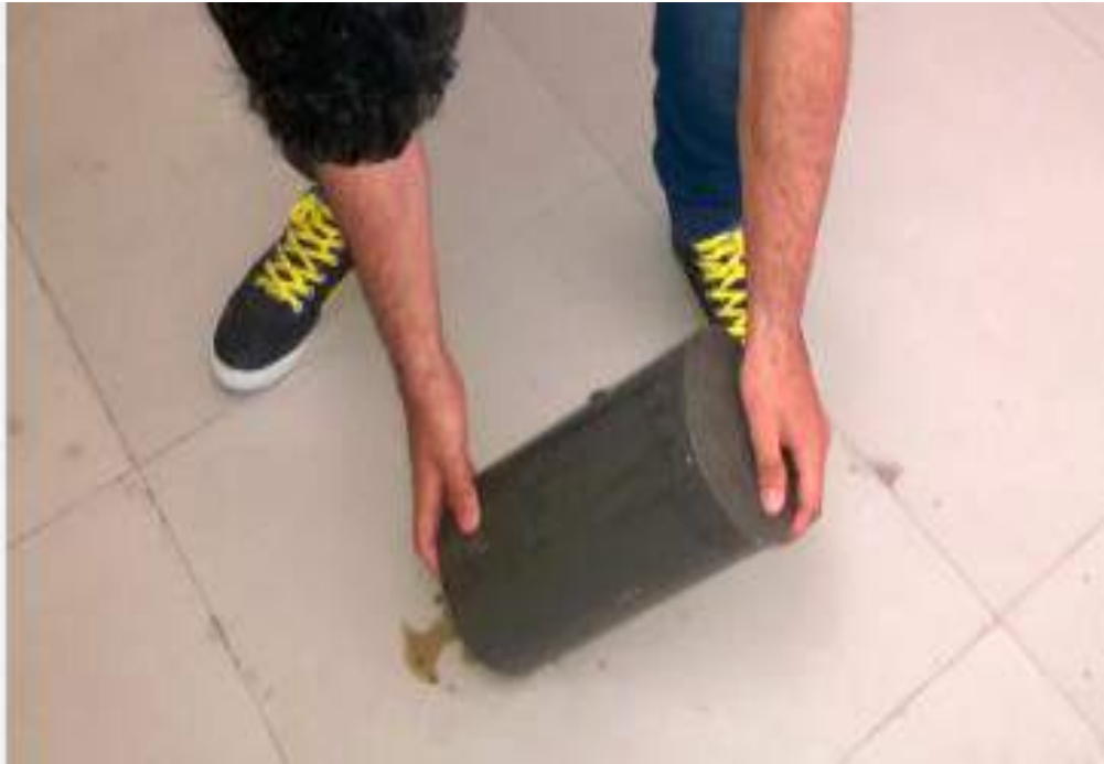
Fig19: Cylindrical concrete specimen after curing of 28days
