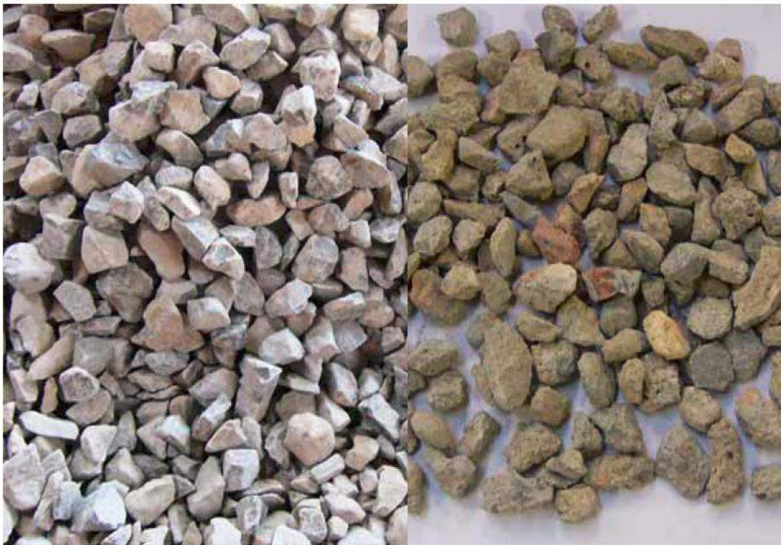
Fig8: Natural aggregates & Recycled aggregates
