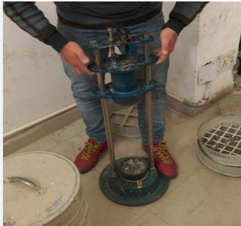
Fig13: Aggregate Impact test (Source: Concrete lab LPU)
