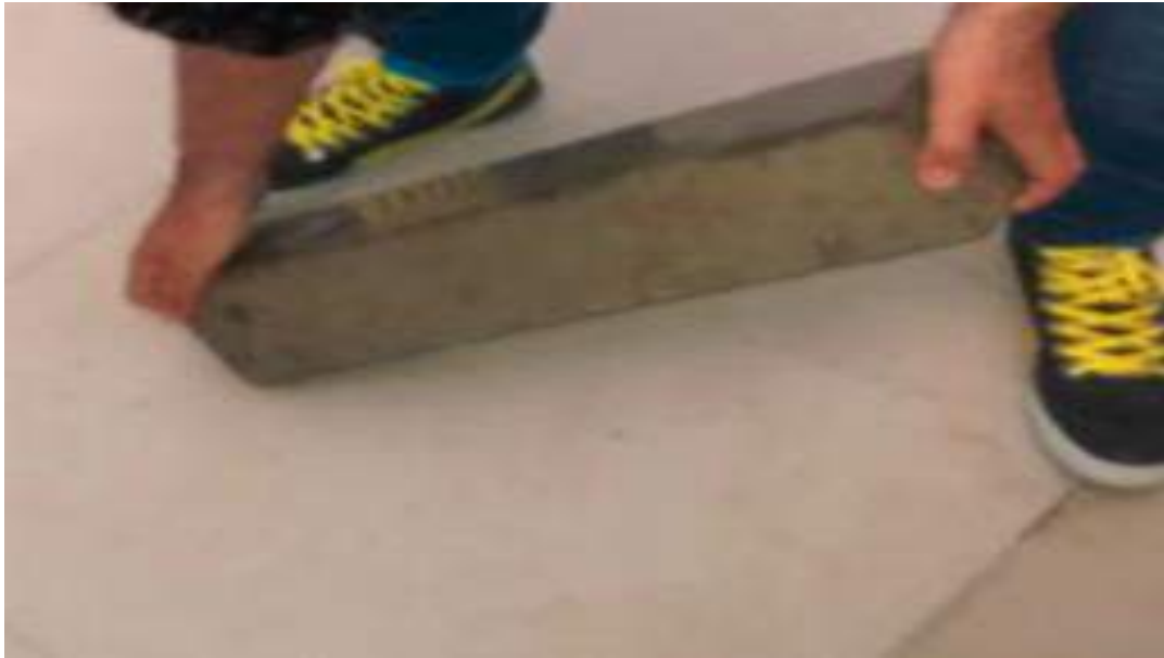
Fig22: Concrete beam after curing of 28days. (Source: Concrete lab LPU)
