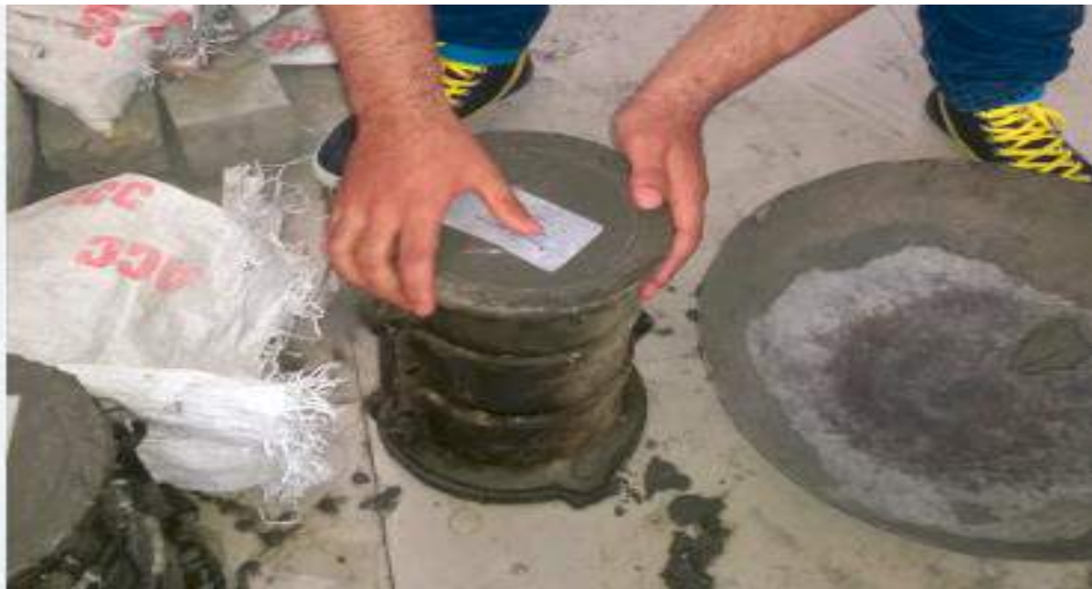
Fig18: Cylinder specimen getting filled by RAC
