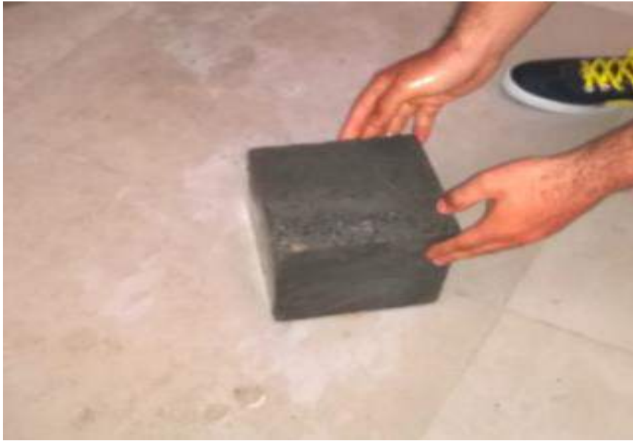
Fig16: Cube after curing of 14days (Source: Concrete lab LPU)
