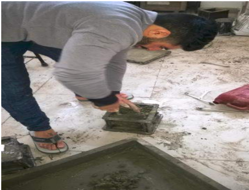
Fig15: filling of RAC in cube (Source: Concrete lab LPU)
