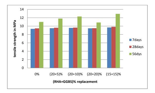
Figure 7.5: Flexural strength of SCC mixes at various ages
