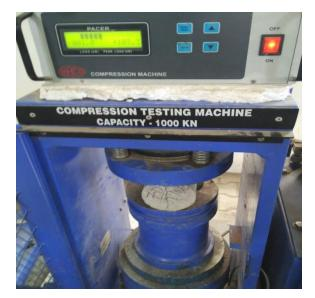
Plate 6.8: Setup for Split tensile strent showing concrete failure
