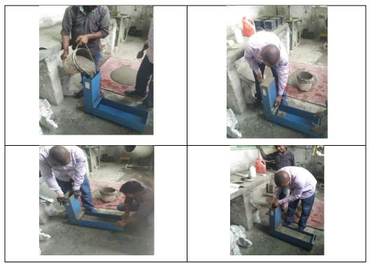
Plate 6.4: L-box test process
