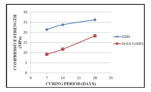
Figure 3.3 Variation of Compressive Strength with Curing period
