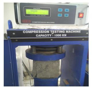
Plate 6.7: Setup for Compressive strength showing concrete failure
