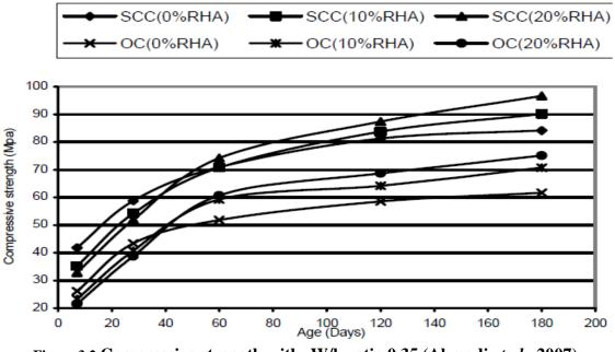
Figure 3.2 Compressive strength with- W/b ratio 0.35 (Ahmadi et al., 2007)
