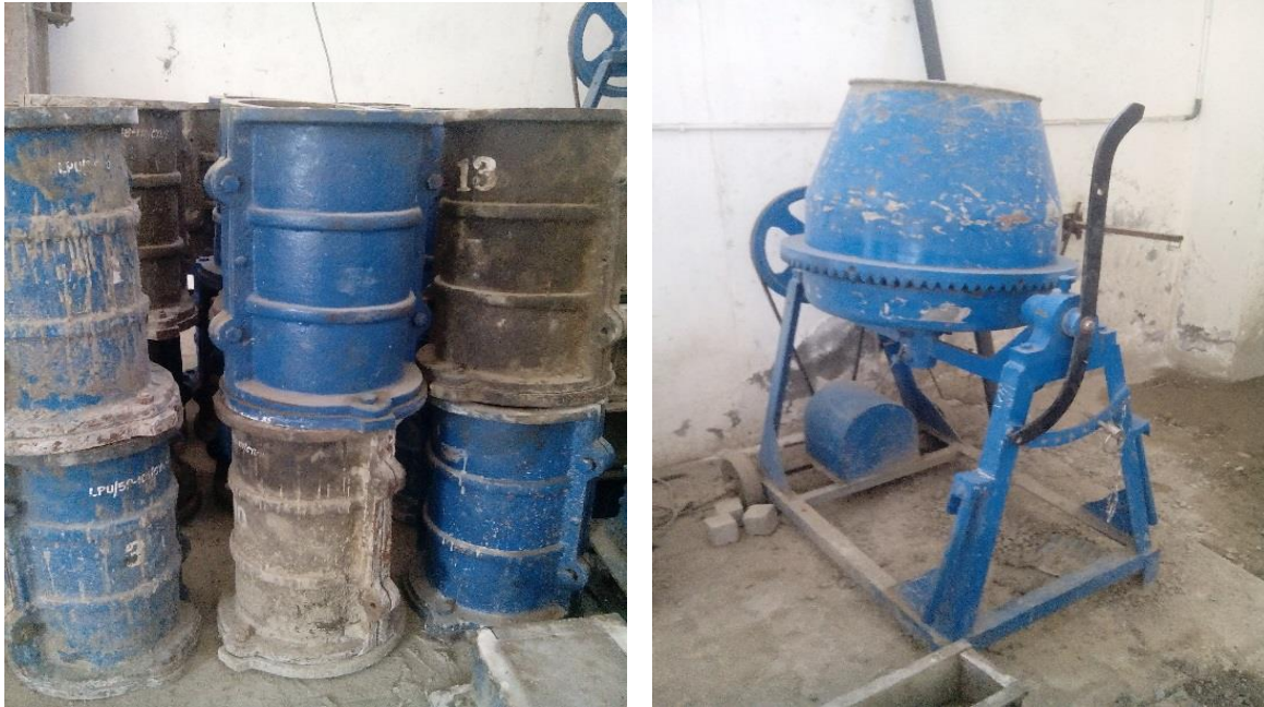
Fig. 7: Picture showing framework of specimens and concrete mixer.
