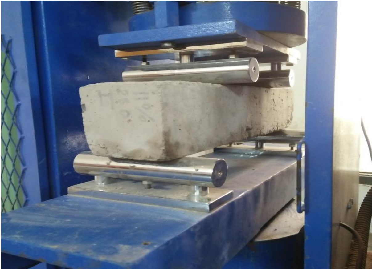
Figure1.6. Flexure test of concrete beam
