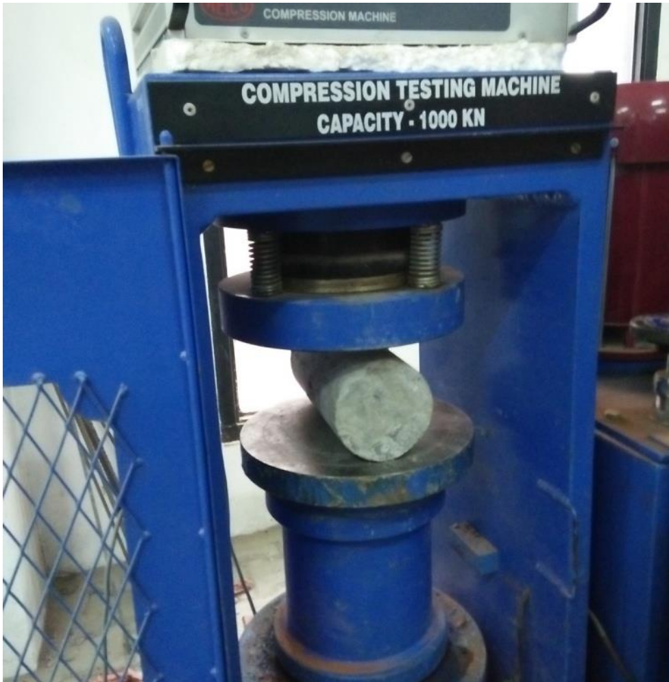
Figure1.5. Split tensile test of concrete cylinder
