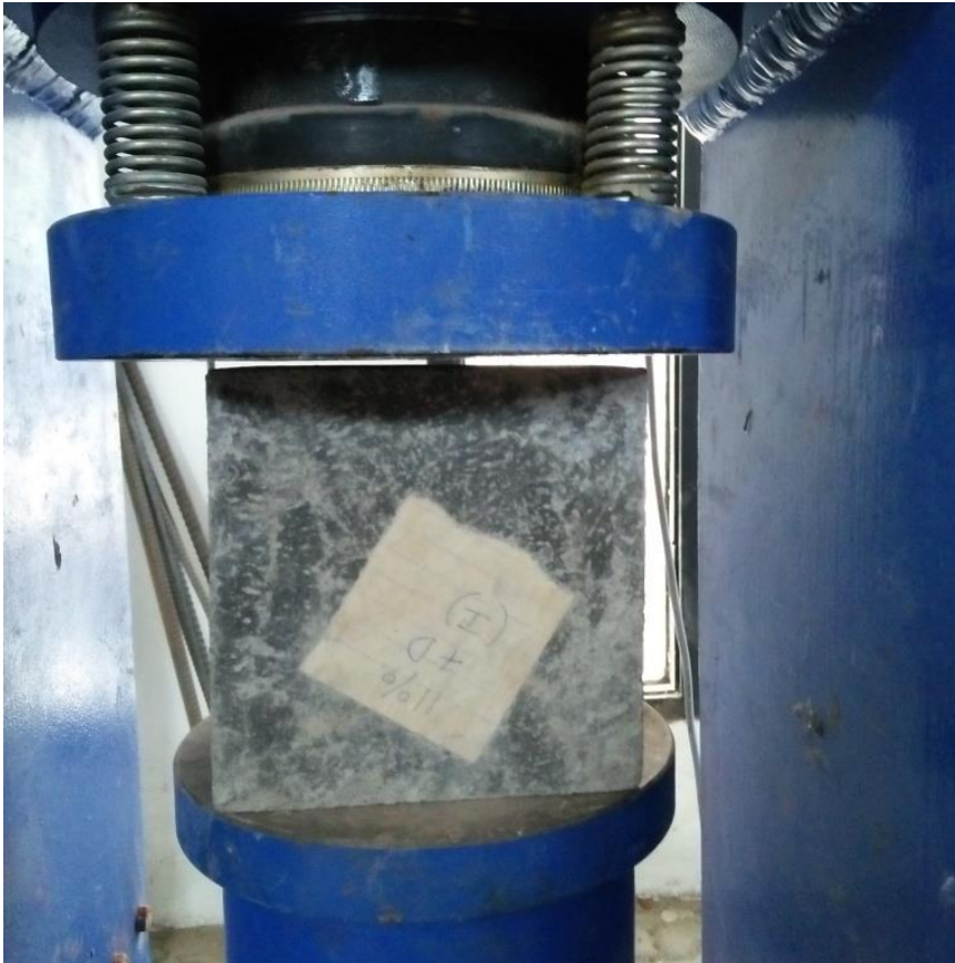
Figure1.4. Compression test of concrete cube
