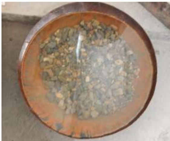
Figure 6.8 water absorption test of coarse aggregate
