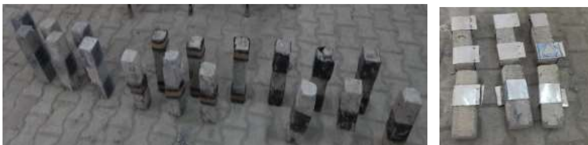
Figure 6.10 Samples with GFRP, elastic tapes, rubber tubes and steel jackets
